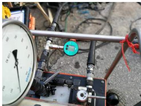
(b) Pressure gauge LEO 3, with dial indicator and compressor
