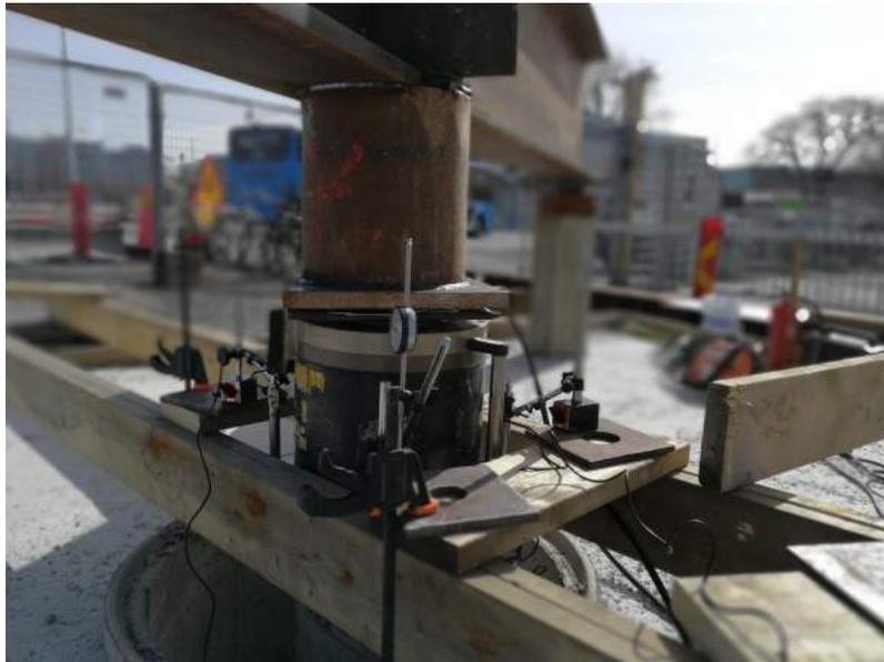
**Figure 3.7:** Dial indicator for pile head movement
