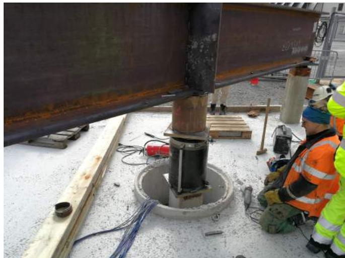
**Figure 3.5:** Hydraulic jack between the test pile and support beams
