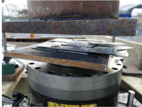
**Figure 6.1:** Skewing of surface between hydraulic jack and supportive beam
