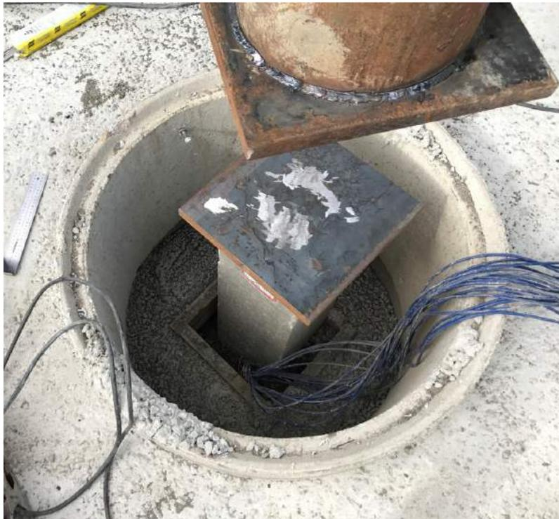
**Figure 3.4:** Footage from the test setup, wooden frame protecting the test pile measuring instruments
