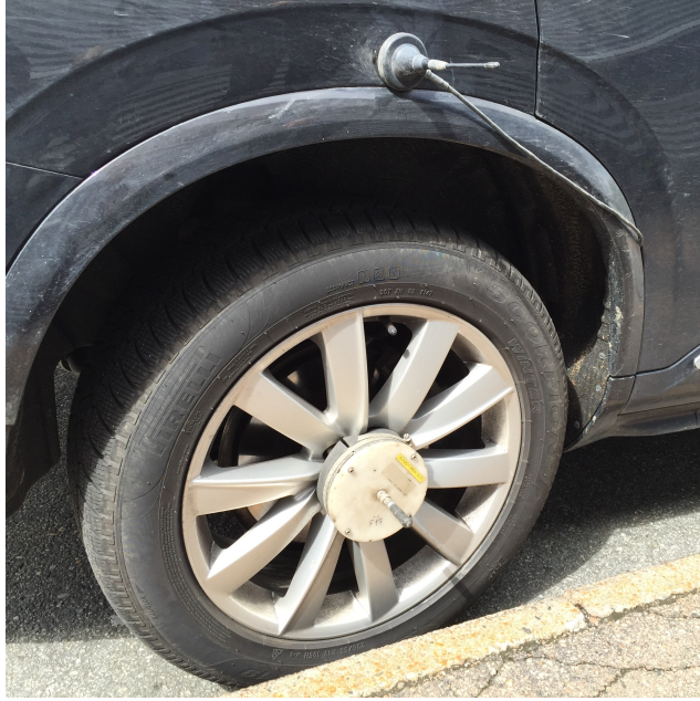
Figure 2.10: Vehicle equipped with sensor for torque measurements
