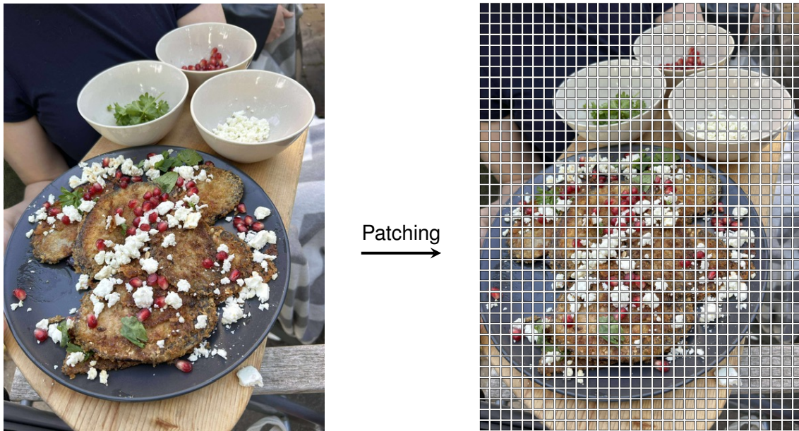
Figure 3.3: When making patches the input image is split into several small and square images with side length determined by the model. For example, DINOv3-Tiny wants squares with side length 14 and DINOv3-Large wants squares with side length 16. In this example, we have an image with size 640 \times 480 and a patch size of 16, giving us 40 \times 30 = 1200 patches of size 16 \times 16 .
