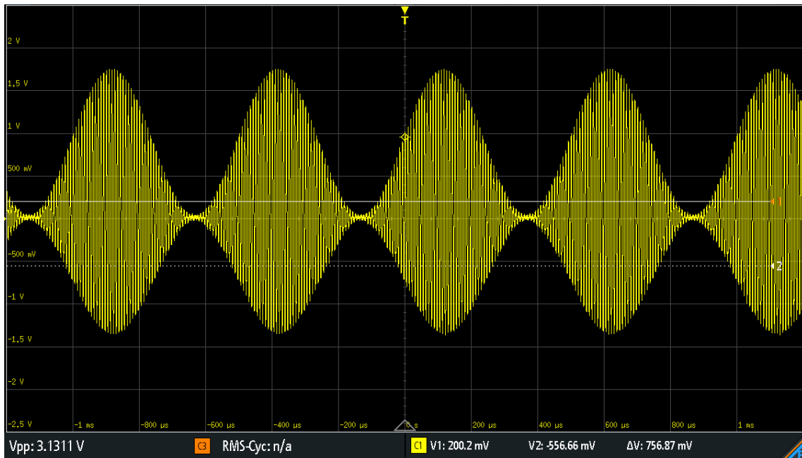
Figure 13. The AM Signal input to the AM demodulator.
