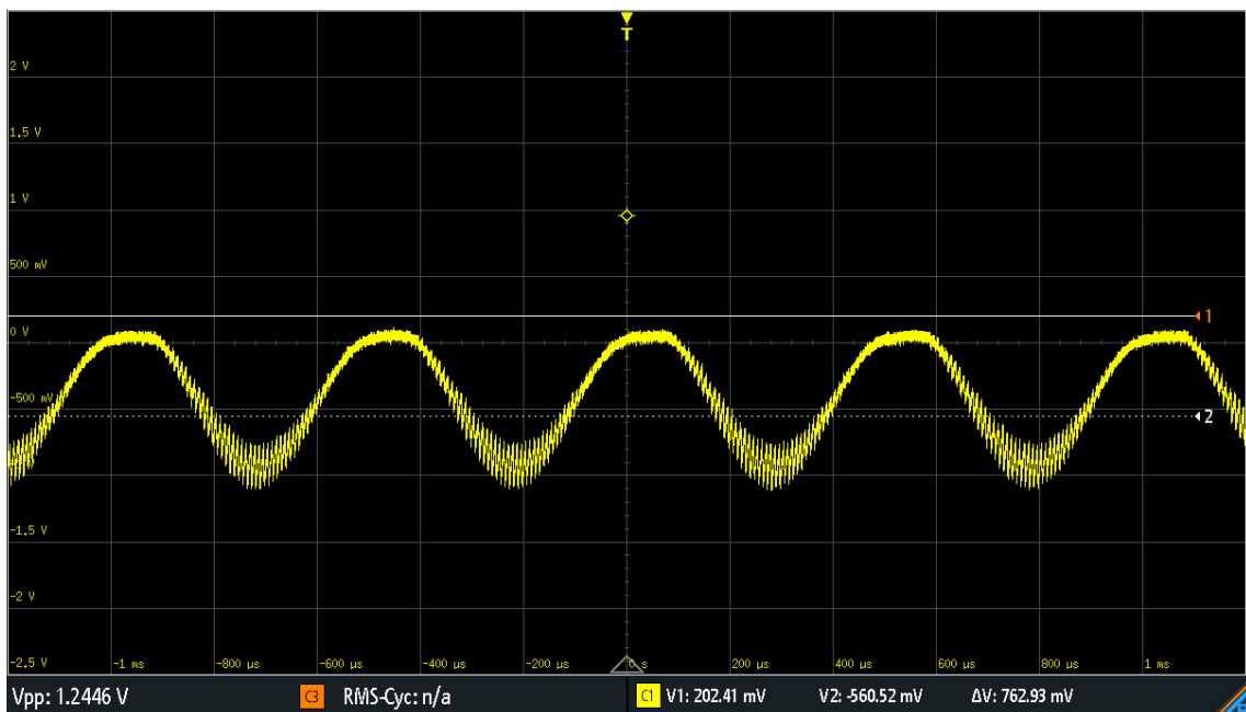
Figure 14. The signal after going through the envelope detector.
