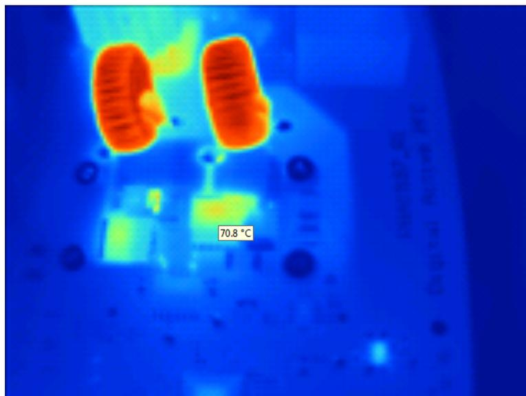
**Figure 4.14:** Thermal close up image of the switches during  $K_f = K_v = 10$ , with maximum transistor casing temperature indicated.
