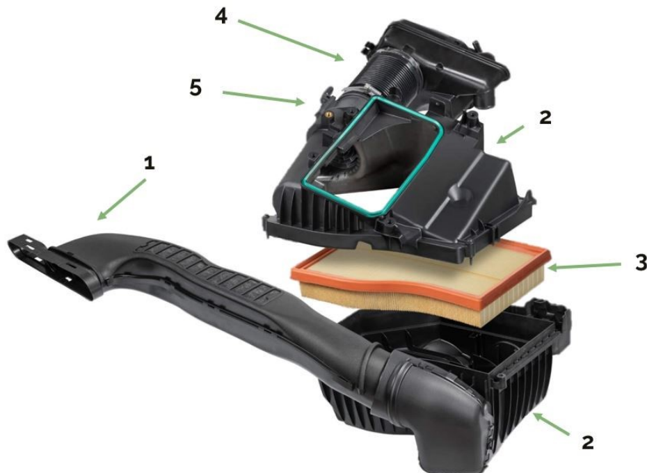
Figure 1.1: Overview of a part of the AIS with the dirty side duct (1), air filter box (2), air filter (3), duct bellow (4), and Mass Airflow Meter (MAF) (5) [1]. With permission from Mann+Hummel.
