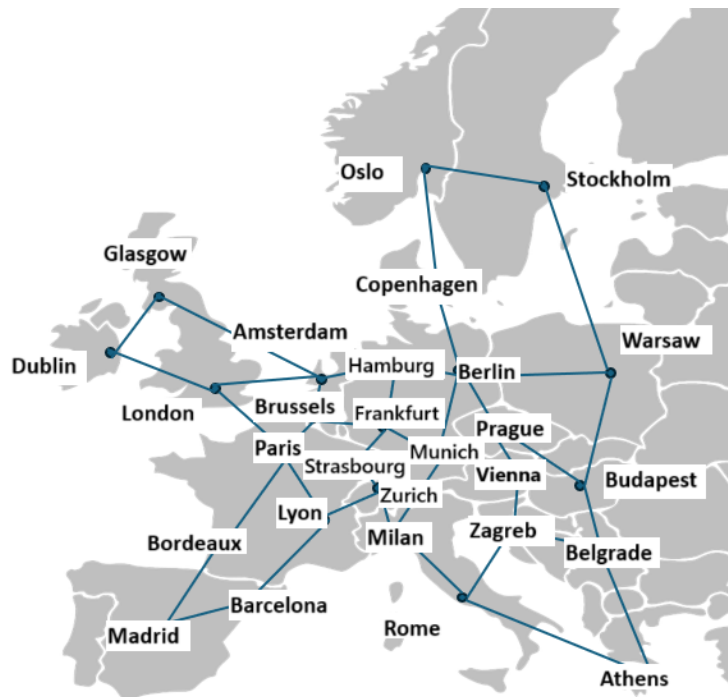
Figure 3.7: EU network topology with 28 nodes and 41 links.
