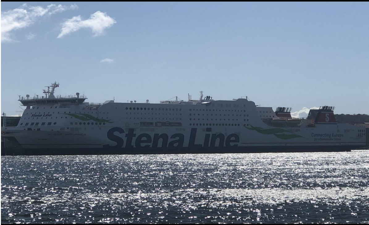
Figure 6: m/s Stena Germanica as she just has arrived in Gothenburg from Kiel. Methanol is used as fuel for the main engines.
