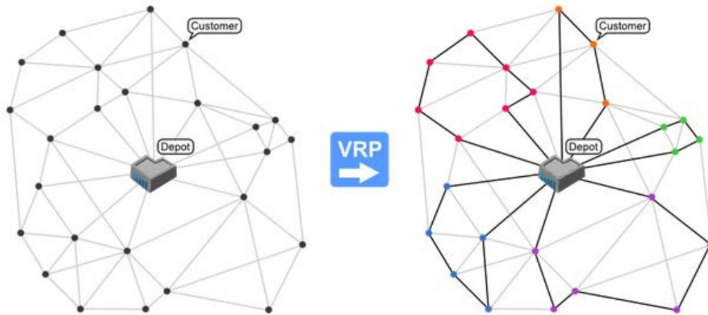
Figure 3.1 - Visualization of the vehicle routing problem
