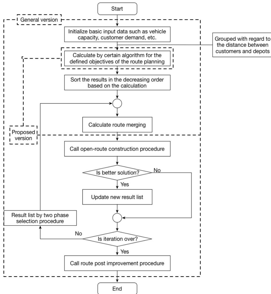
Figure 3.11 - Flowchart for Software Route planning
