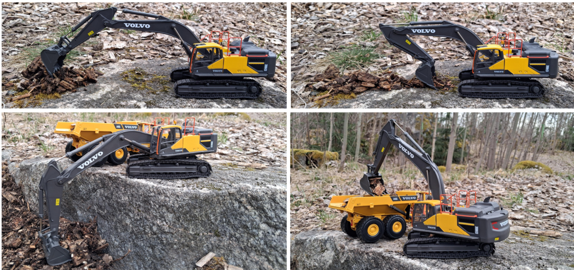
Figure 3.2: Examples of excavator operations. The two upper images show a grading action and the two lower images show a dig-and-dump action.
