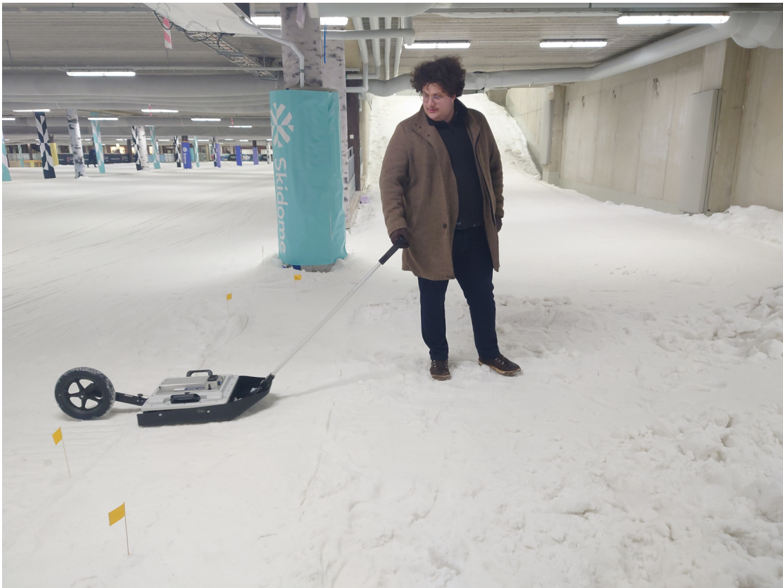
Figure 3.11: Gathering data with MALÅ GPR at Skidome
