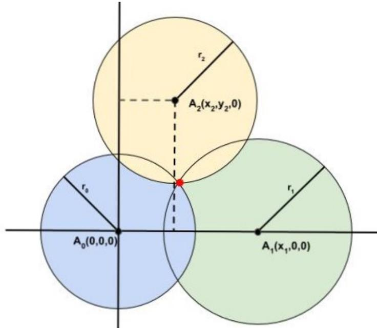
**Figure 2.4:** Trilateration with three anchors.
