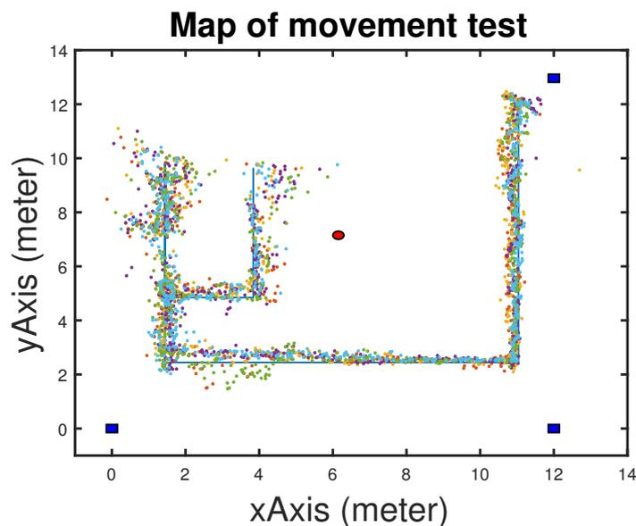
**Figure 5.8:** The sampling points during the large scale (slow) position test plotted along with the course, concrete pillar and the anchors.
