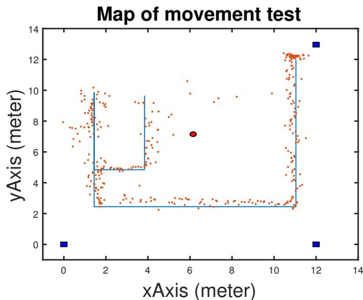
**Figure 5.13:** The sampling points during the large scale (pocket) position test plotted along with the course, concrete pillar and the anchors.
