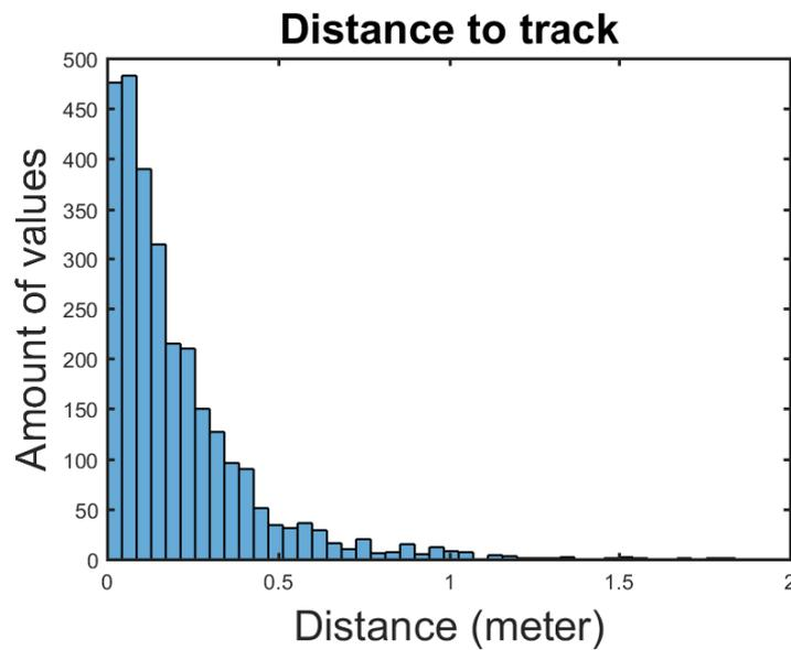
**Figure 5.10:** Histogram of distance deviation from the course during large scale (slow) position test for the full test.
