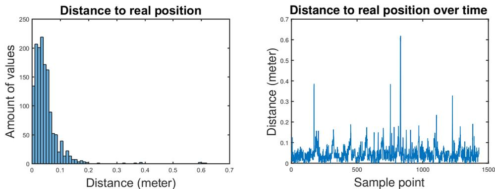
**Figure 5.7:** Results from the small scale position test, presented as a histogram and as a function of time.
