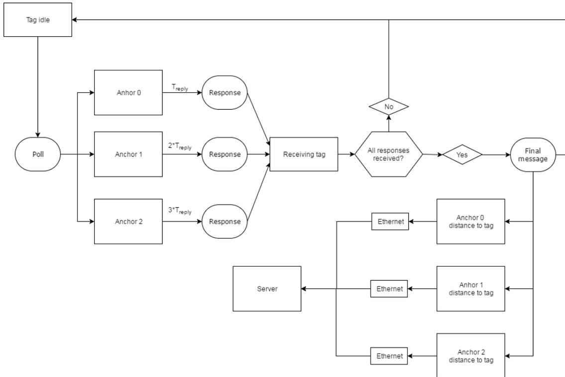
**Figure 4.2:** A flowchart describing the positioning of one tag
