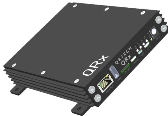
**Figure 4.3:** Picture of the QRx made by QRTECH which is used as anchor.
