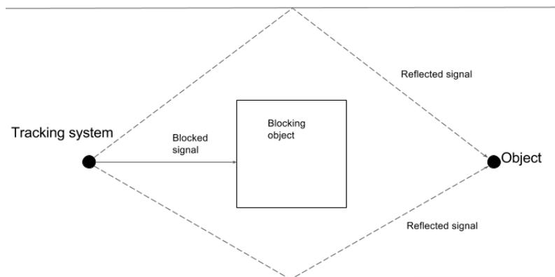
**Figure 2.1:** Communication between system and target with an object blocking the sight between them.
