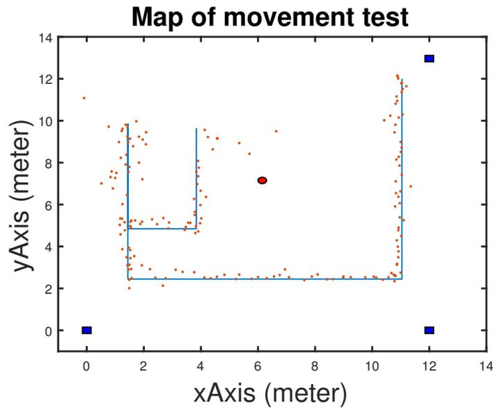
**Figure 5.12:** The sampling points during the large scale (fast) position test plotted along with the course, concrete pillar and the anchors.
