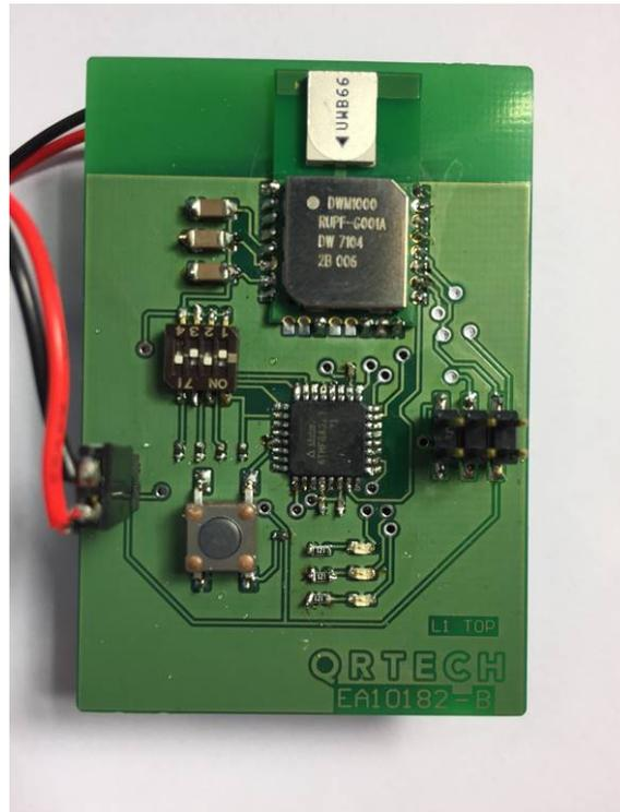
**Figure 4.4:** Picture of the custom made PCB used as a tag.
