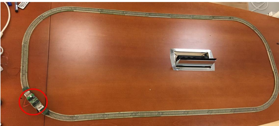
**Figure 5.5:** Test environment used during the test, an electronic miniature railway with length of 464 centimeters with tag attached on train shown in the circle.
