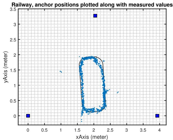
**Figure 5.6:** The sampling points during the small scale position test plotted along with the railway and the anchors.
