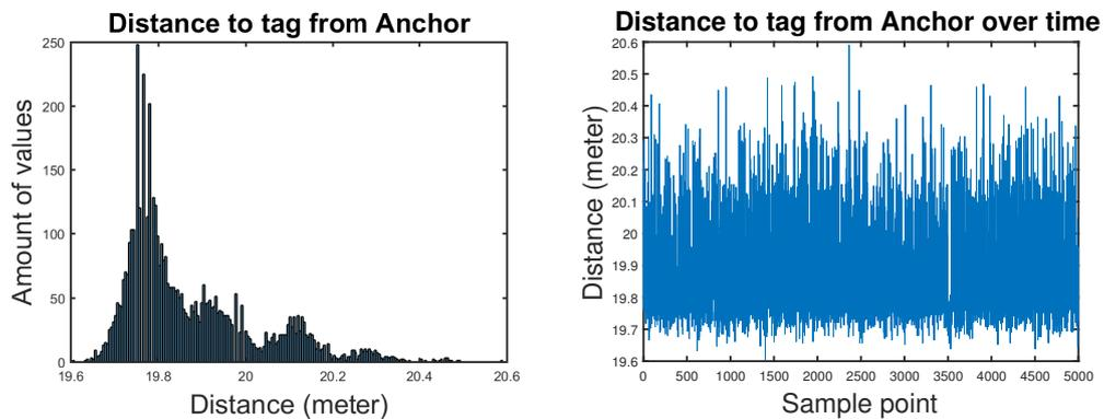
**Figure 5.4:** Results from the 20 meter test, presented in a histogram and as a function of time.
