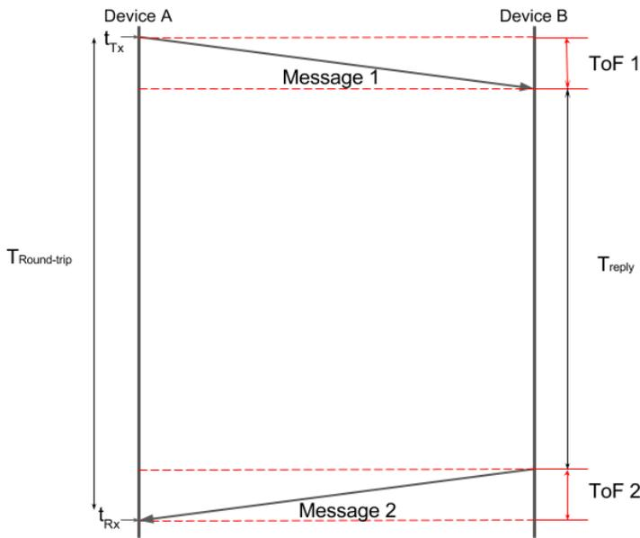
**Figure 2.2:** Message structure for ToF measurement.
