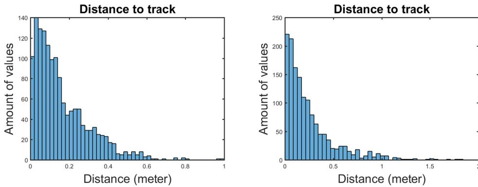
**Figure 5.9:** Histogram of distance deviation from the course during large scale (slow) position test for first half (left) of the course and second half (right).
