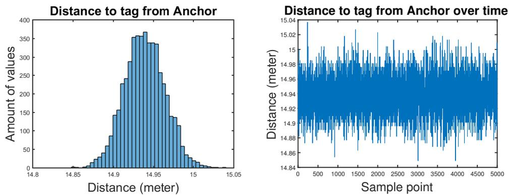
**Figure 5.3:** Results from the 15 meter test, presented in a histogram and as a function of time.
