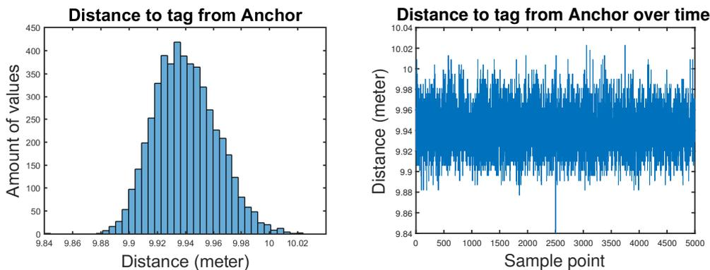
**Figure 5.2:** Results from the 10 meter test, presented in a histogram and as a function of time.
