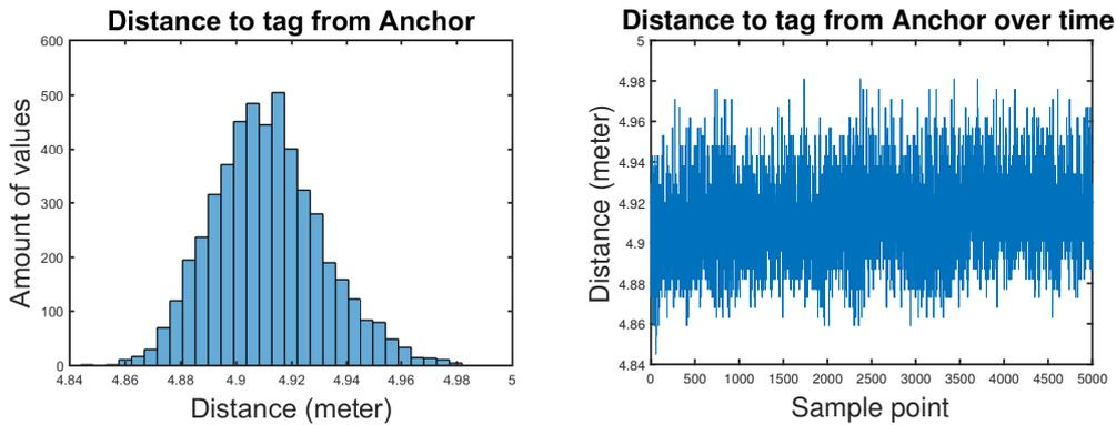
**Figure 5.1:** Results from the 5 meter test, presented in a histogram and as a function of time.
