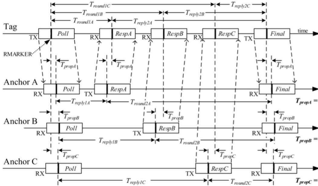
**Figure 4.6:** Two way ranging with three anchors and one tag with a poll message [28].
