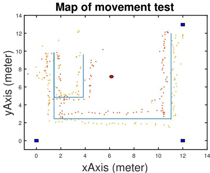
**Figure 5.14:** The sampling points during the large scale (multiple tags) position test plotted along with the course, concrete pillar and the anchors.
