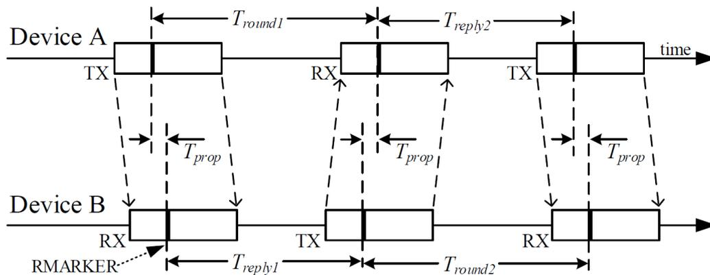
**Figure 2.3:** Double-sided ToF message structure [28].
