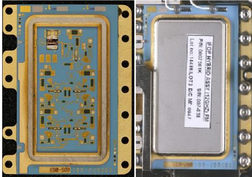
Figure 6. Example of packaged LTCC hybrid. Left: the hybrid circuit, inside of package. Right: packaged. (picture not correct according to scale)
