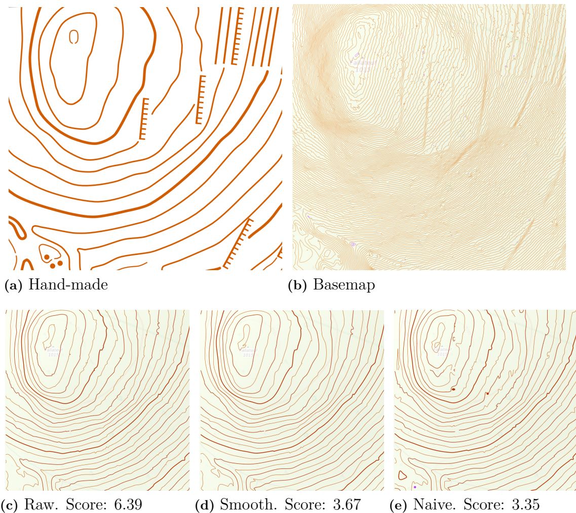
Figure 5.3: As expected do the generated contours quite will on smooth steep hills as steep hills means that the contours are close together. The earth banks from the hand-made map are quite prominent in the basemap, but neither of the methods do a good job showing them by bending the contours upwards. The smooth contours exaggerate the edge where the left most earth bank is located the best.
