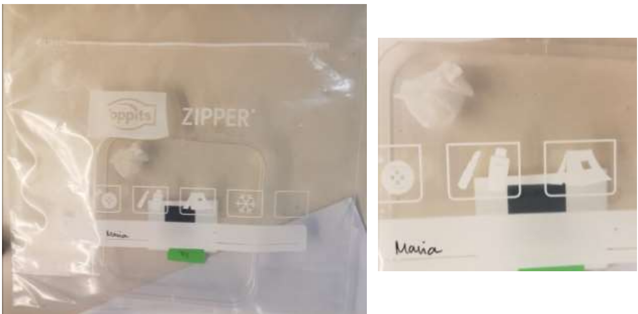
Figure 6: Sample environment with filter paper. Left picture presents the experimental setup and the right one is a zoomed in to visualize the saturated environment and the filter paper closer.
