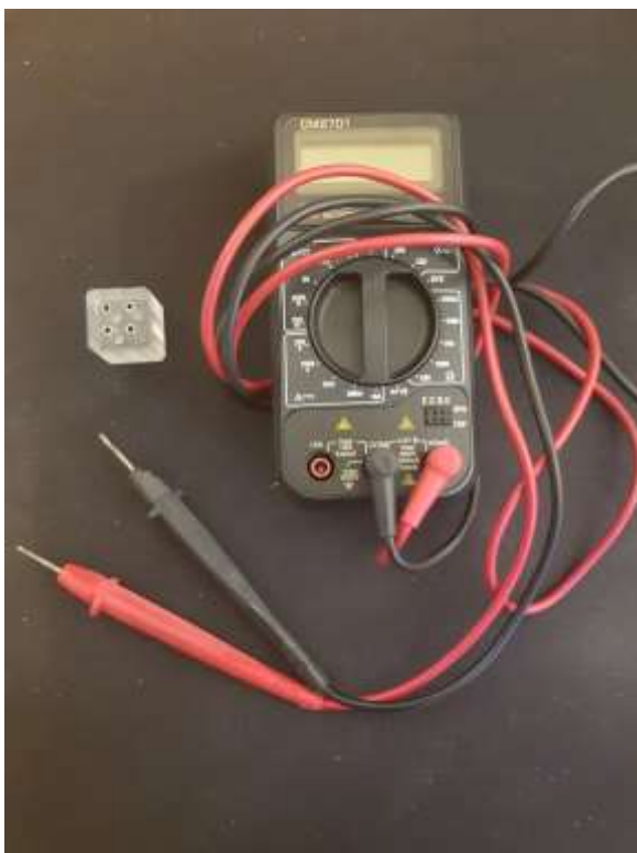
Figure 7: Left picture is an overview of the resistance measurement strategy device. The little box made of plexiglass and the multimeter with adjusted probes to establish a fixed distance of 8 mm. Right picture is a zoom in picture of the plexiglass box, top and bottom.
