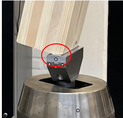
Figure 3-29 The connection between a specimen and the hydraulic press clamp.
