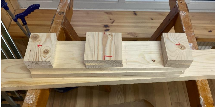
Figure 3-6 Longitudinal layers and cross-layers ready for production of a specimen.
