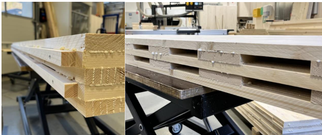
Figure 4-6 Timber elements at the edges of the cross-layers (left) and the CLT panel after disassembly (right).
