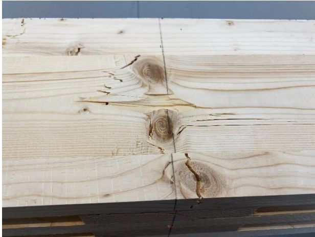
Figure 4-61 Tensile failure at the bottom of Sample 1.
