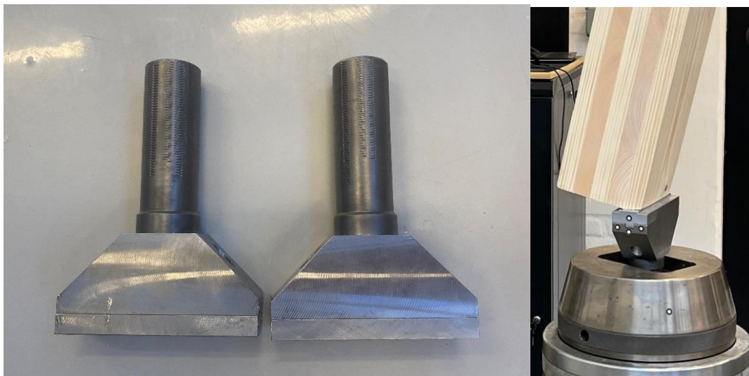
Figure 3-18 Fixtures and the steel plates.
