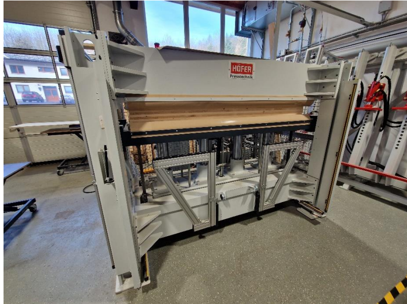
Figure 4-5 Hydraulic press and the pressing process.
