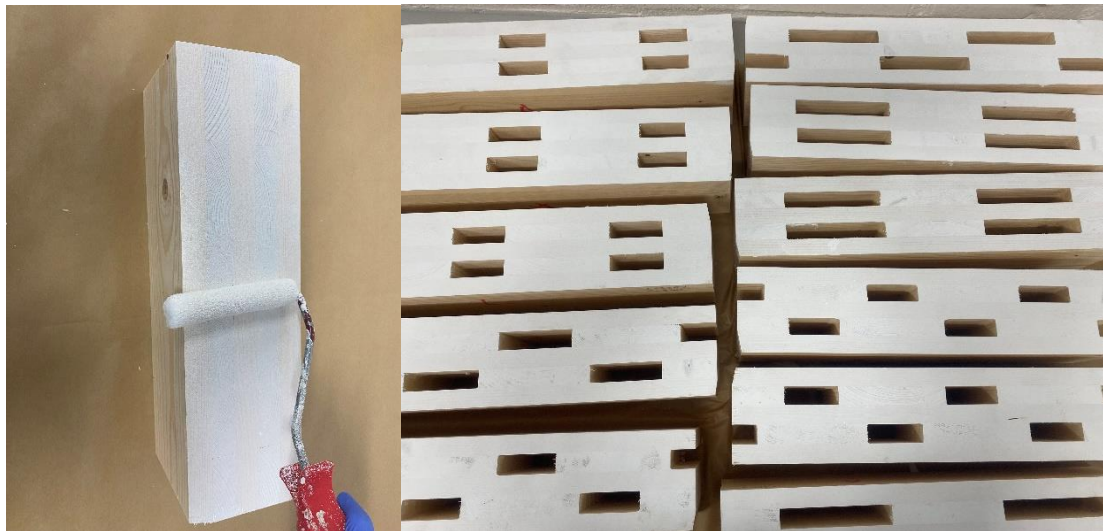
Figure 3-15 The process of covering the specimens with white paint.
