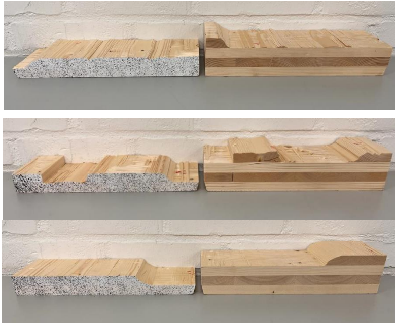
Figure 3-37 Detailed results from the shear test of Configuration I, with the order from top to bottom, Sample 1, Sample 2, and Sample 3, respectively.
