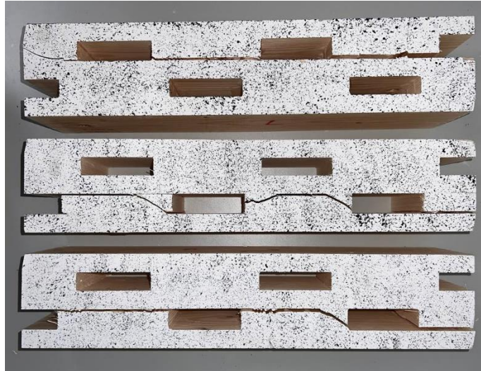
Figure 3-69 Shear test results of Configuration VI, with the order from top to bottom, Sample 1, Sample 2, and Sample 3, respectively.
