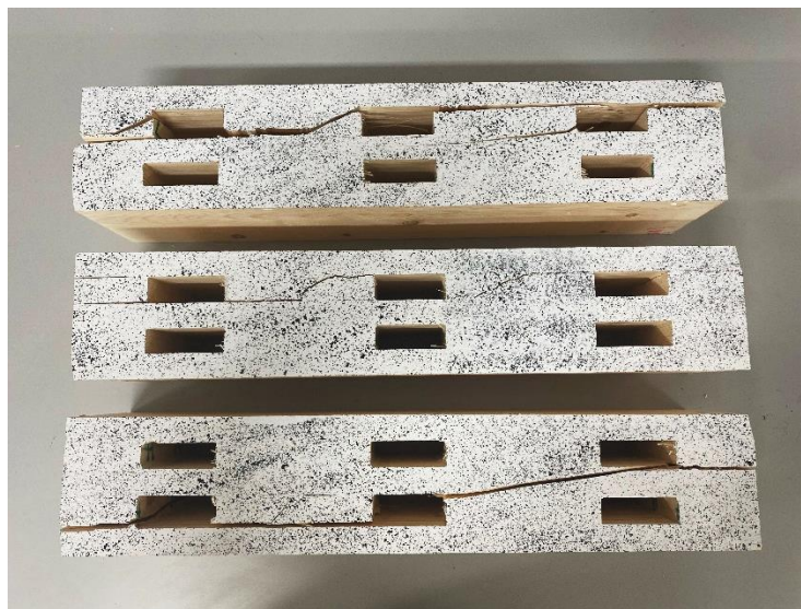
Figure 3-110 Shear test results of extra samples of Configuration II, with the order from top to bottom, Sample 4, Sample 5, and Sample 6, respectively.
