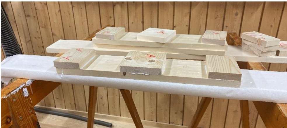
Figure 3-9 Gluing of the cross-layers.
