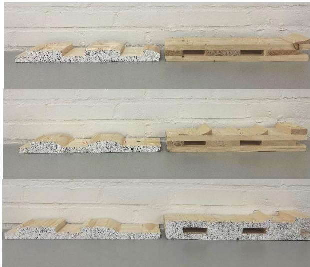
Figure 3-70 Detailed results from the shear test of Configuration VI, with the order from top to bottom, Sample 1, Sample 2, and Sample 3, respectively.
