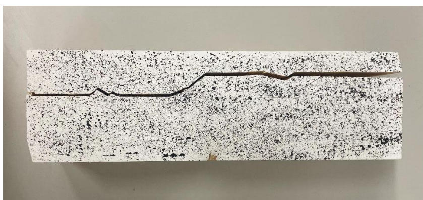
Figure 3-104 Shear test results of an extra sample of Configuration I.
