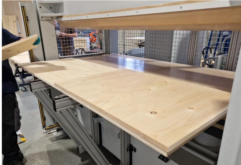
Figure 4-3 Manual assembling of the cross-layer boards.
