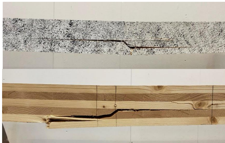
Figure 4-31 Detailed pictures of the failure for Sample 3 of Configuration A. The picture at the top depicts the front side, and the bottom one shows the unpainted backside of the beam.
