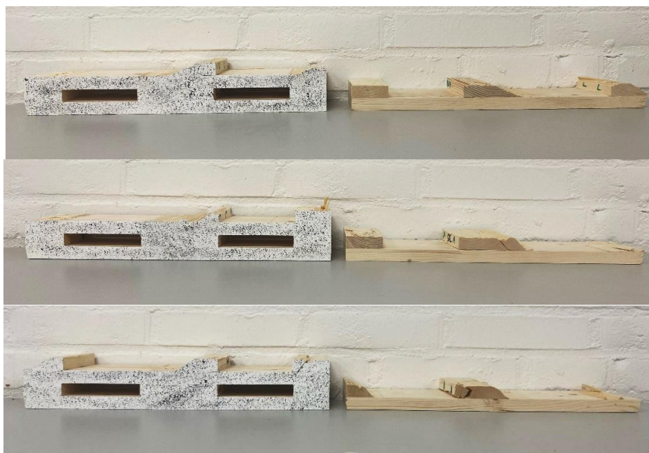
Figure 3-122 Detailed results from the shear test of extra samples of Configuration IV, with the order from top to bottom, Sample 1, Sample 2, and Sample 3, respectively.
