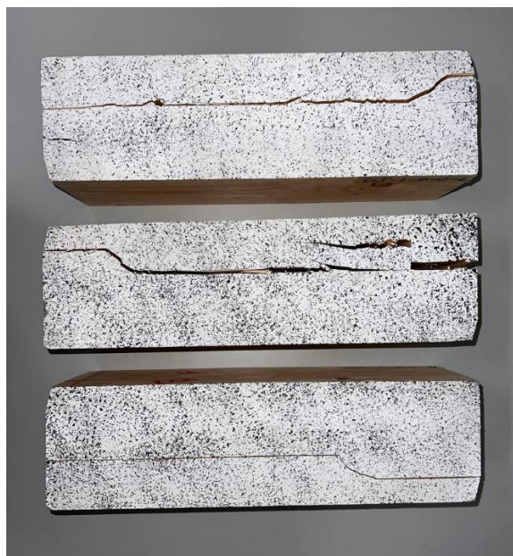
Figure 3-36 Shear test results of Configuration I, with the order from top to bottom, Sample 1, Sample 2, and Sample 3, respectively.
