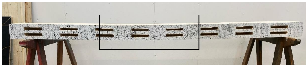
Figure 4-59 Test results and failure mode of Sample 1 of Configuration C. The black rectangle shows the location of the failure.
