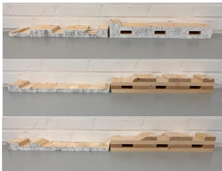
Figure 3-43 Detailed results from the shear test of Configuration II, with the order from top to bottom, Sample 1, Sample 2, and Sample 3, respectively.
