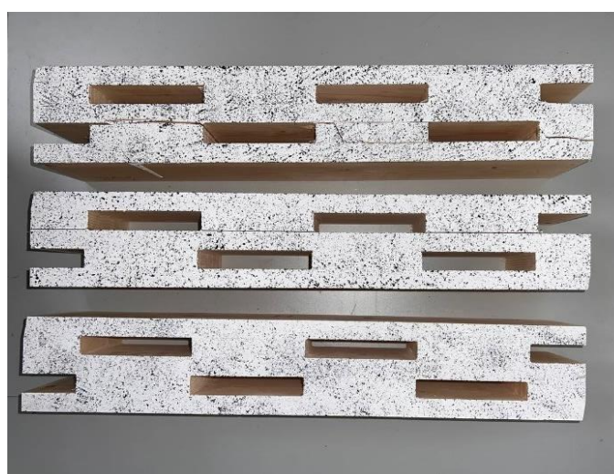
Figure 3-61 Shear test results of Configuration V, with the order from top to bottom, Sample 1, Sample 2, and Sample 3, respectively.
