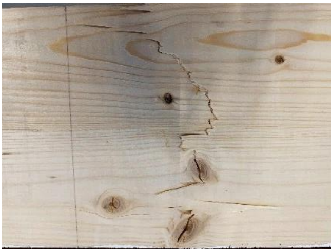
Figure 4-64 Tensile failure at the bottom of the Sample 2.
