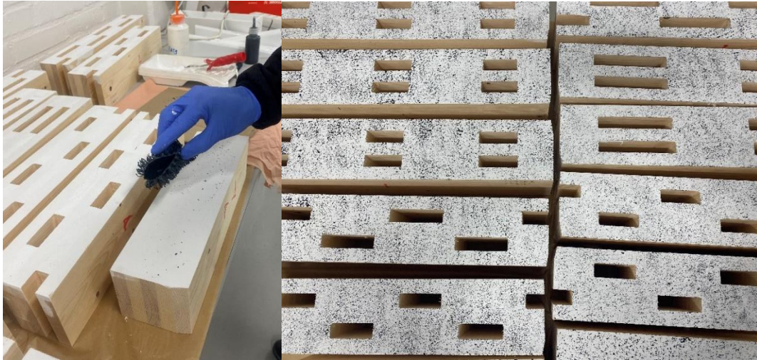
Figure 3-16 Covering the specimens with the pattern.
