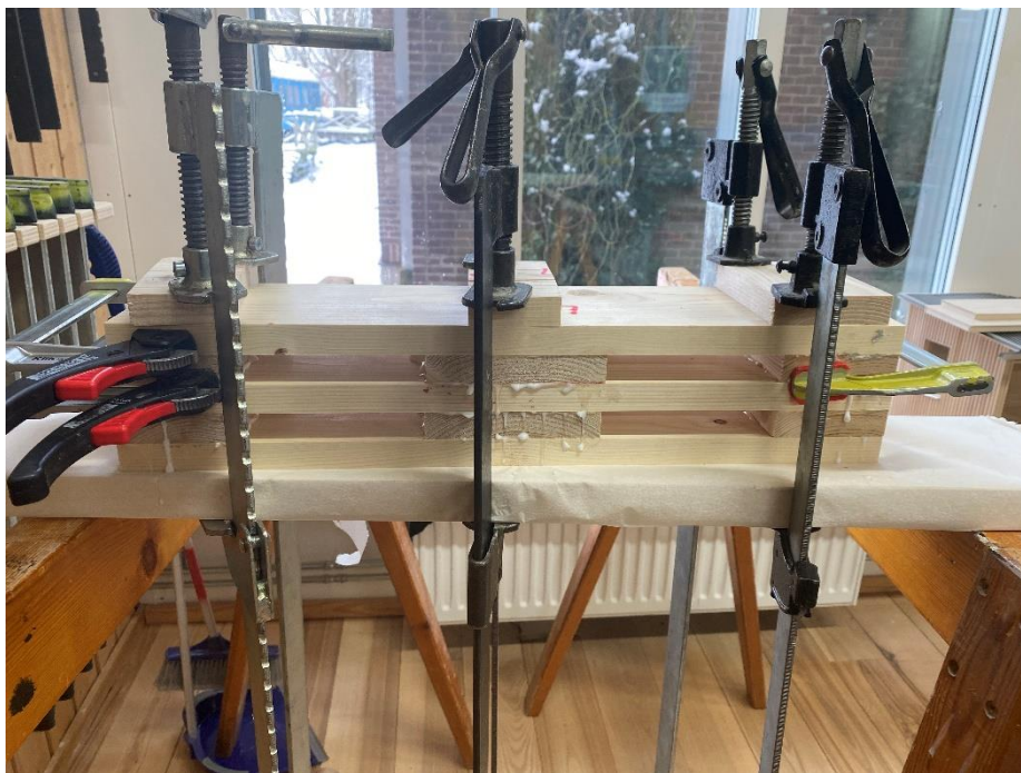
Figure 3-11 The final clamping and drying of the specimen.
