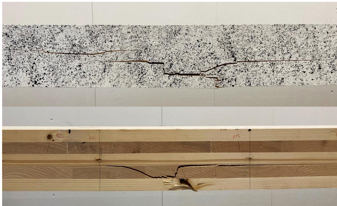
Figure 4-27 Detailed pictures of the failure for Sample 1 of Configuration A. The picture at the top depicts the front side, and the bottom one shows the unpainted backside of the beam.
