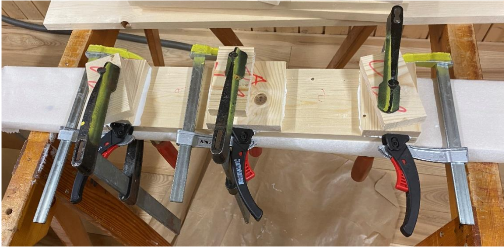
Figure 3-10 Clamping the first and second layers to prevent sliding of the cross-layers.
