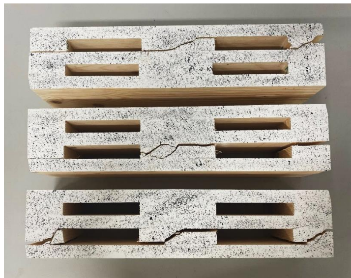
Figure 3-121 Shear test results of extra samples of Configuration IV, with the order from top to bottom, Sample 1, Sample 2, and Sample 3, respectively.
