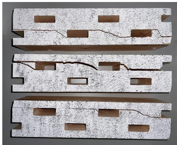
Figure 3-49 Shear test results of Configuration III, with the order from top to bottom, Sample 1, Sample 2, and Sample 3, respectively
