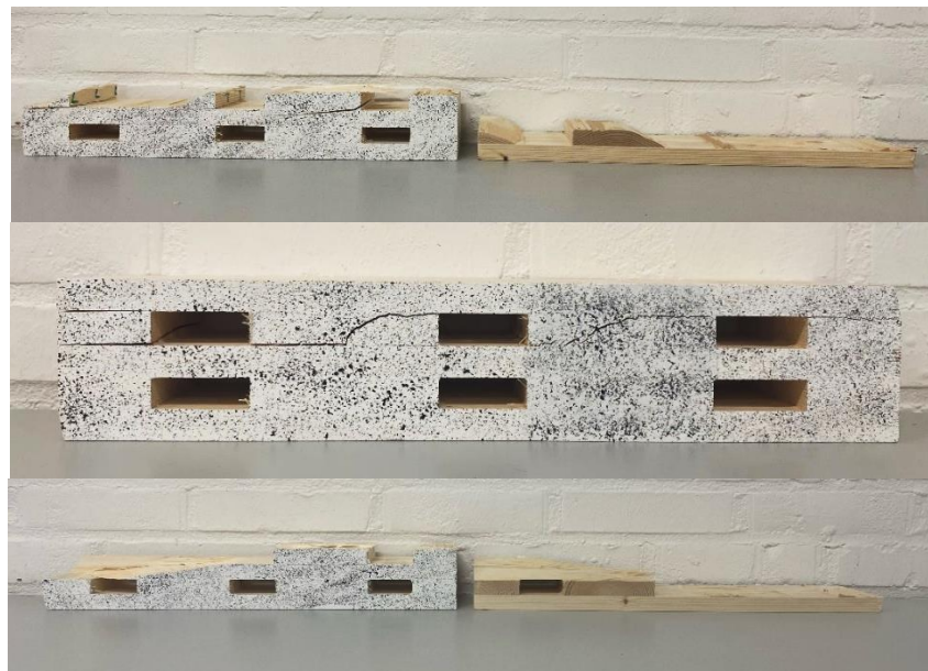
Figure 3-111 Detailed results from the shear test of extra samples of Configuration II, with the order from top to bottom, Sample 4, Sample 5, and Sample 6, respectively.
