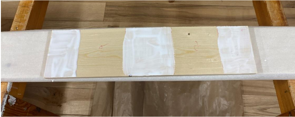
Figure 3-8 The spread of the glue at the longitudinal layer where the cross-layers will be placed.
