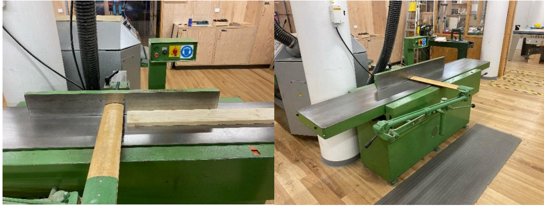
Figure 3-4 The planing machine and the planing process along the width of the board.
