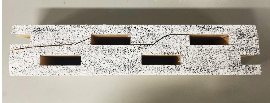
Figure 3-130 Shear test results of an extra sample of Configuration VI.
