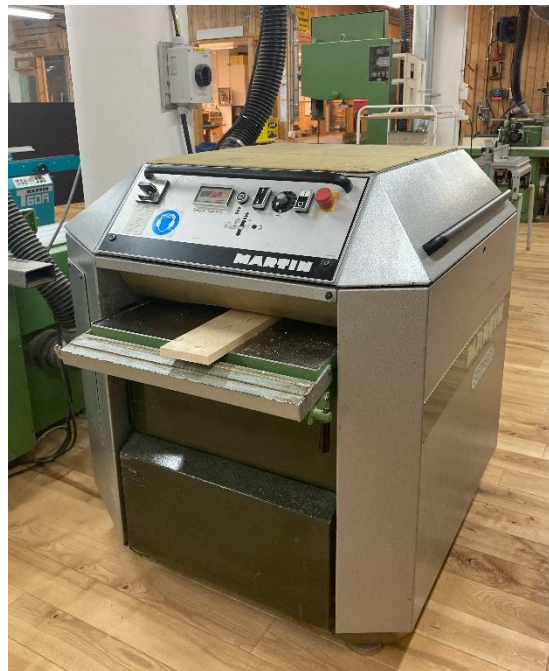
Figure 3-5 Planing machines used for obtaining desired thickness.
