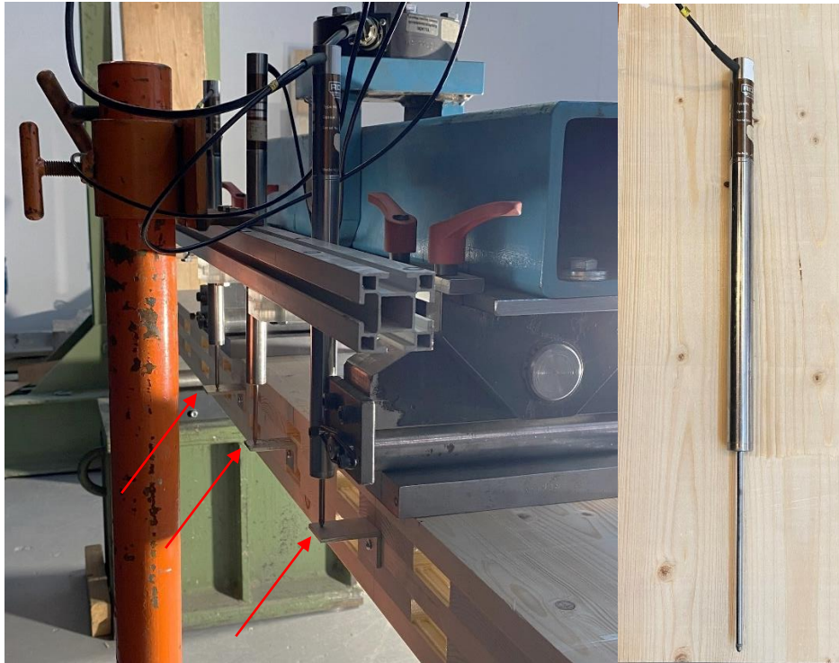
Figure 4-13 The location of sensors behind the beam.
