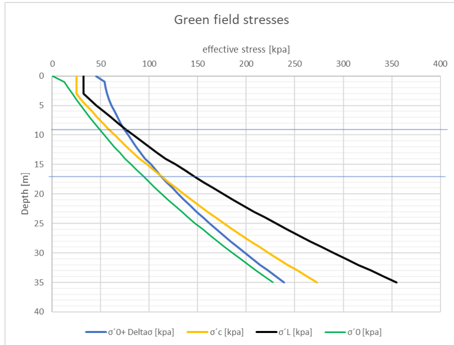
Figure 3.3: Green Field effective stress distribution versus depth, The blue lines determine the different cases for settlement calculation following Swedish method
