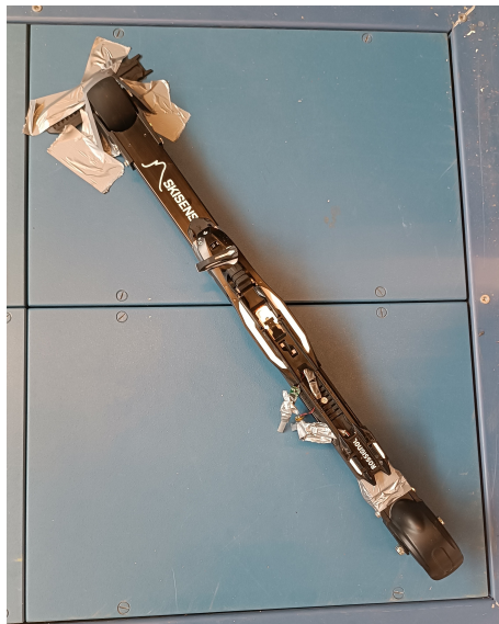
Figure 4.6: Test of the prototype mount on a roller ski on the force plate
