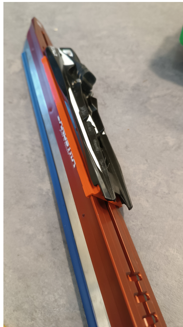
Figure 5.1: Binding prototype mounted on recreational ice skate
