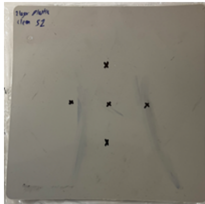
Figure 3.5: Thickness measuring points
