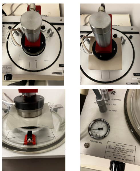
Figure 3.6: illustration of placing sample inside test cell
