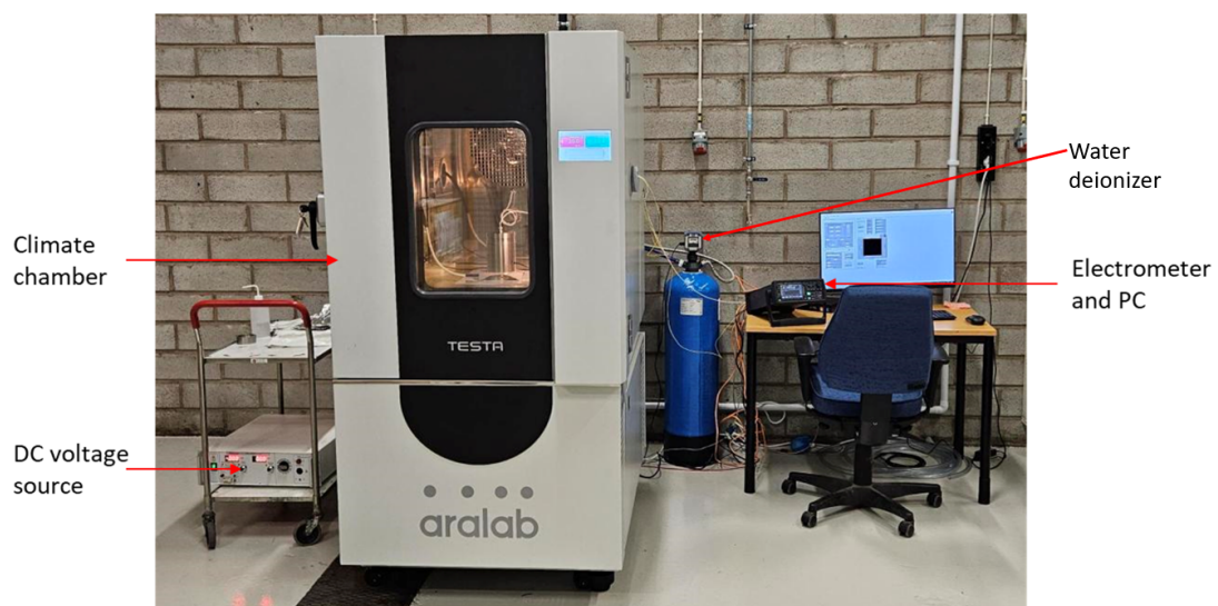
Figure 3.7: Overview of PDC measuring setup
