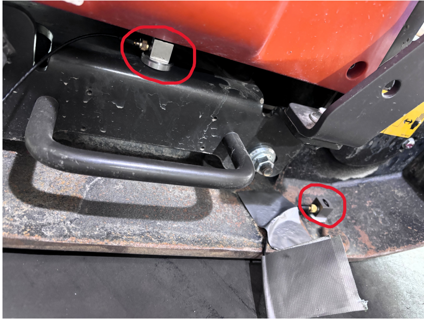
Figure 4.1: Accelerometers mounted on the bottom plate and the frame of the plate compactor.
