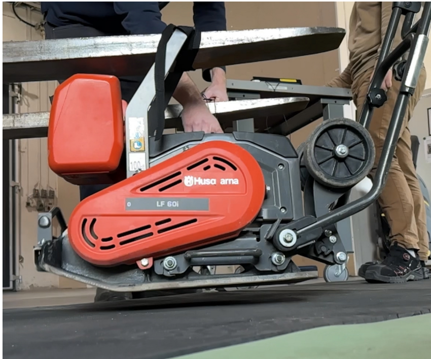
Figure 4.2: Plate compactor suspended in the frame.
