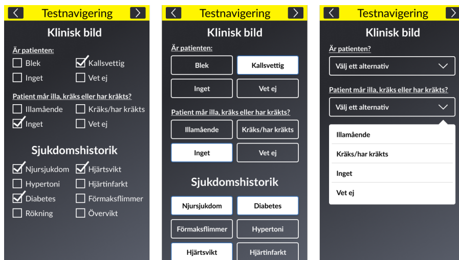
Figure 23 - Screens for different input methods for picking options. From left: checkboxes, buttons, dropdown menu.
