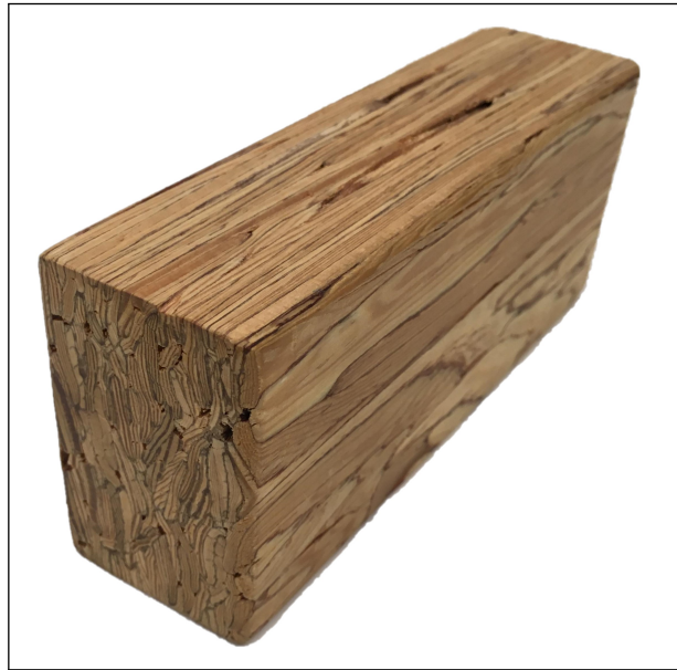
Figure 2.4: Small specimen showing the structure of PSL.
