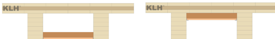
Figure 3.3: Two different ways of how to utilise the space between the ribs. Images © KLH / Rib Elements Version 09/2019
