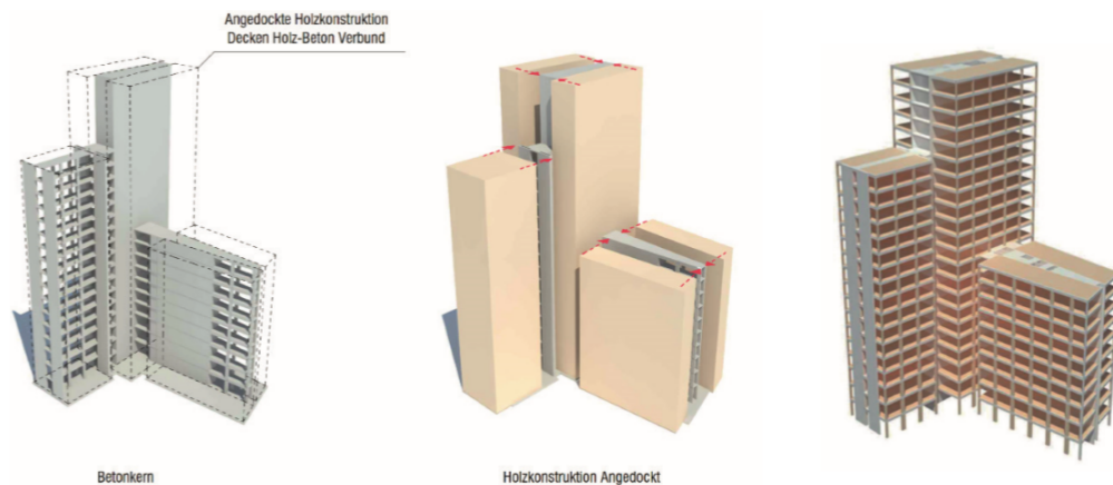
Figure 4.5: Illustration of the structural concept in HoHo Vienna. A timber hybrid structure that is attached to a concrete core (Woschitz and Zotter, 2017). Images © RWT plus ZT GmbH
