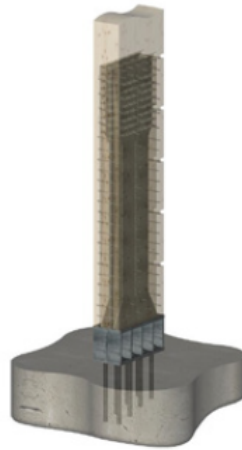
Figure 4.10: Detail of how the CLT shear walls are connected to the foundation (Cecobois, 2018). Image © Nordic Structures / www.nordic.ca
