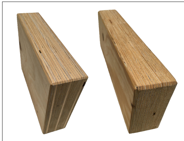
Figure 2.3: Two smaller pieces of LVL. The left have three layers with the fibres perpendicular, while the right have all layers in the same direction.
