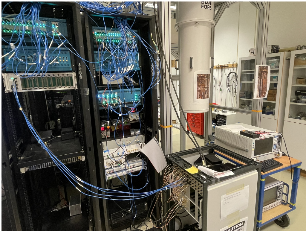
Figure 3.6: This picture shows the setup in the lab. On the right, the white cylinder is the dilution fridge. Below (in the picture), the SPI-rack is located. The QBlox clusters are the blue boxes in the top part of the racks on the left of the picture.
