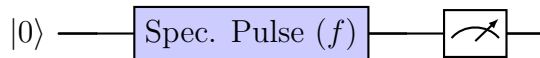
Figure 4.3: Pulse sequence for qubit spectroscopy. The qubit is first initialized to the ground state |0\rangle by relaxing the qubit. A spectroscopy pulse with variable frequency f is applied to drive the qubit transition |0\rangle \rightarrow |1\rangle . Finally, the qubit state is measured by probing the readout resonator. This sequence is repeated over a range of frequencies to identify the qubit transition frequency by detecting the resonance condition where the spectroscopy pulse excites the qubit.
