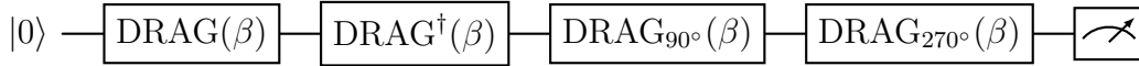
Figure 4.9: Pulse sequence for Motzoi (DRAG) parameter calibration. After letting the qubit relax to |0\rangle , a series of DRAG pulses with quadrature correction \beta are applied, including standard and inverse pairs to enhance sensitivity to leakage. For |0\rangle \rightarrow |1\rangle calibration, additional phase-shifted pulses ( 90^\circ and 270^\circ ) are included to detect subtle leakage paths. The qubit is then measured to extract population dynamics as a function of \beta , enabling fine-tuning of the DRAG coefficient for optimal leakage suppression.
