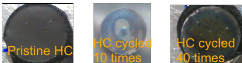
**Figure 4.26:** Photo taken of two electrodes cycled in full cell setups showing a bluish tone as compared to the pristine electrodes.
