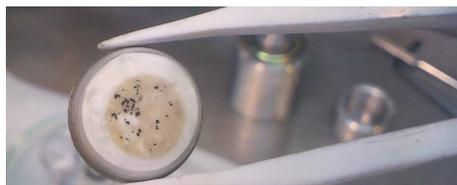
**Figure 4.29:** Separator showing HC disintegration after cycling.
