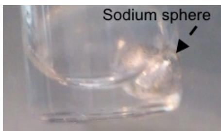
**Figure 4.3:** A Na sphere stored with 1 M  $\text{NaPF}_6$  in diglyme
