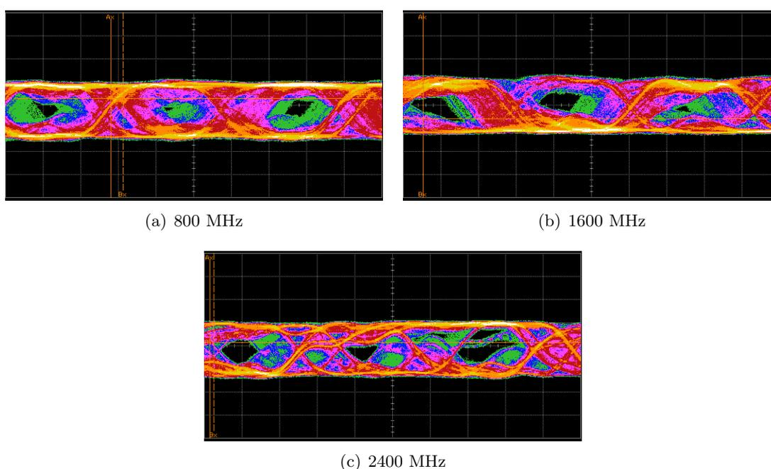
Figure 5.16.: Output from the baseband for different intermediate frequencies.
