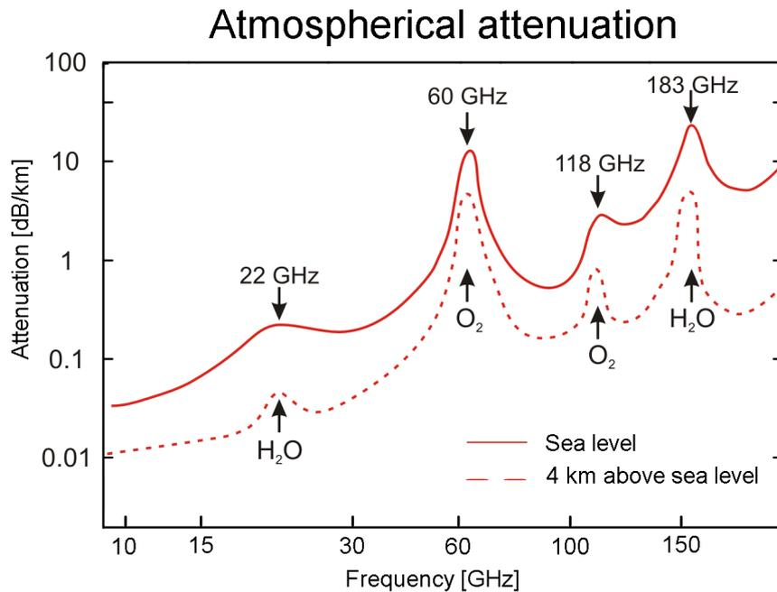
Figure 1.1.: The atmospherical attenuation of radio signals for different frequencies.
