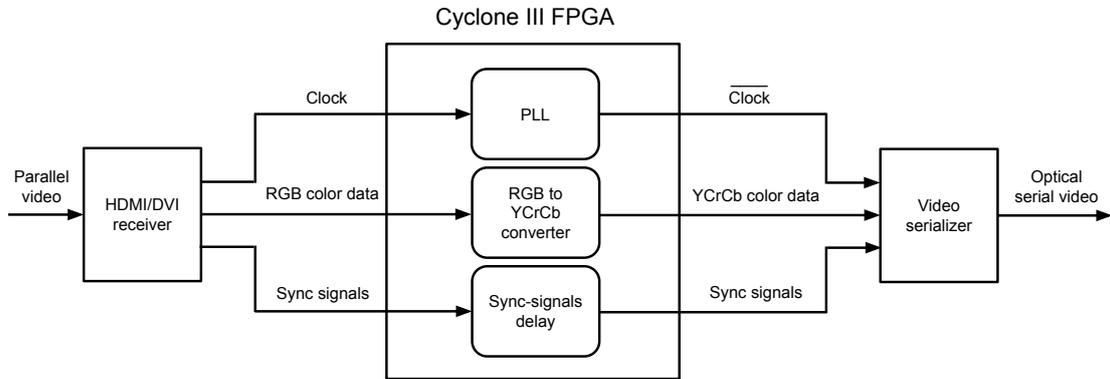
Figure 4.4.: Overview of the FPGA design for video processing on the transmitter side.
