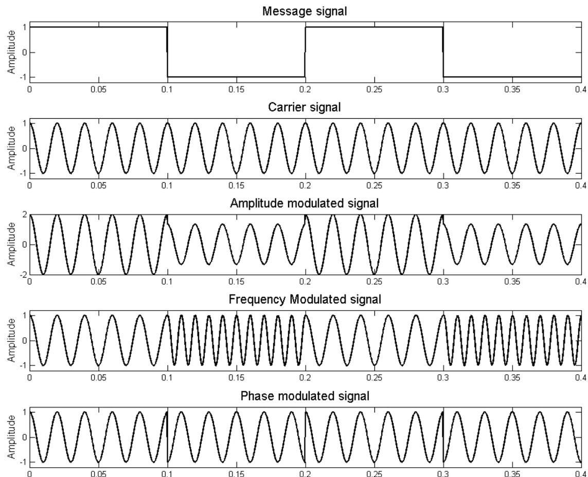
Figure 3.2.: Basic analog modulation techniques.
