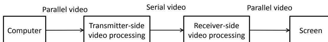
Figure 5.6.: Video test setup with the Cyclone III platforms.
