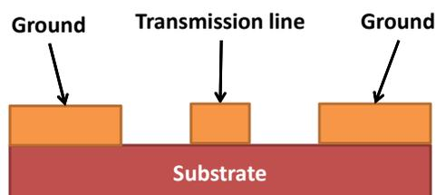
Figure 4.9.: Cross-section of a grounded coplanar waveguide.
