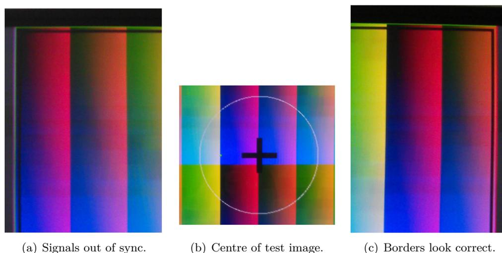
Figure 5.5.: Three test image outputs from the video system.
