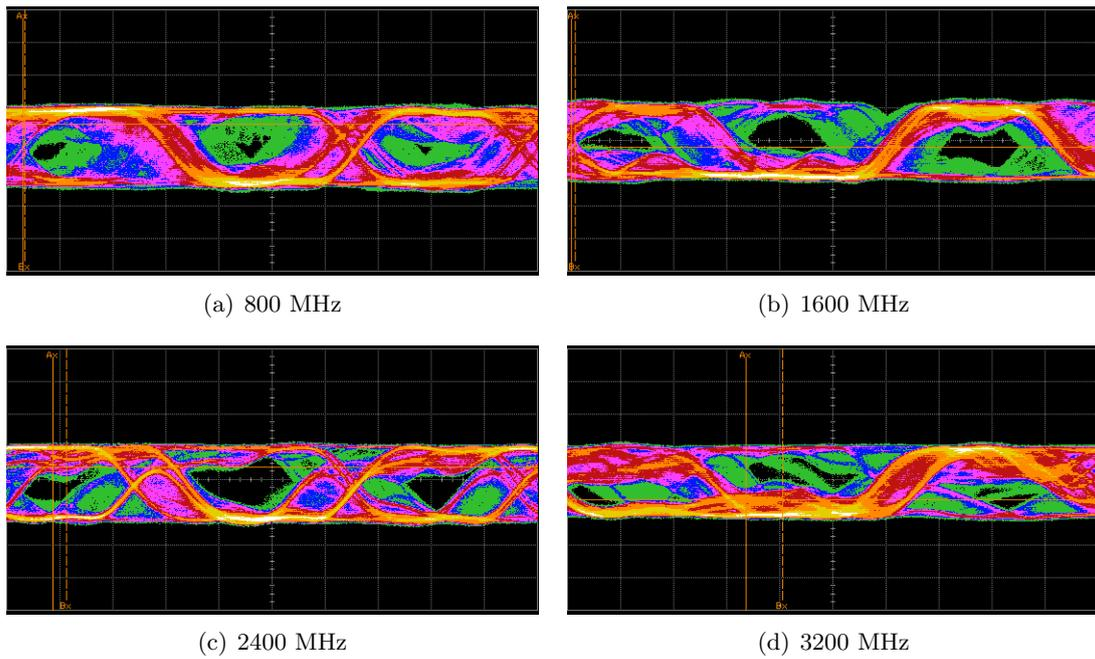
Figure 5.17.: Output from the baseband with terminated inputs for different intermediate frequencies.
