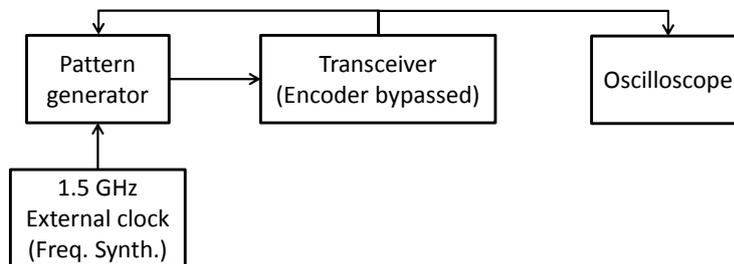
Figure 5.7.: Block diagram of the cyclone IV GX transceiver test setup.
