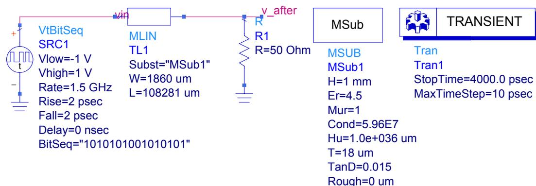
Figure 4.16.: The simulation setup in ADS for the transient analysis.
