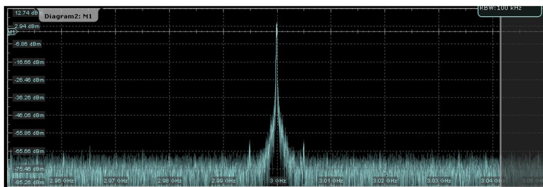
Figure 5.12.: The output signal generated by the frequency synthesizer.
