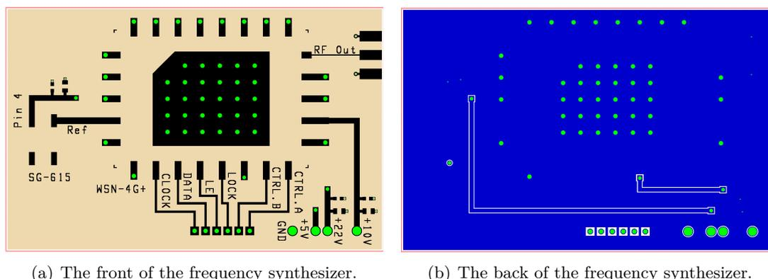
Figure 4.14.: The front and back of the frequency synthesizer.
