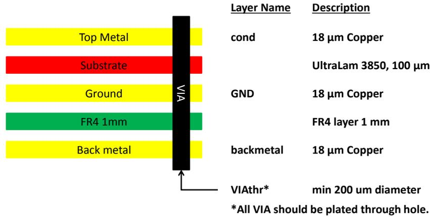
Figure 4.10.: The design stack for the PCBs.
