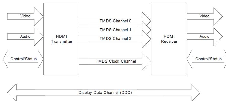
Figure 3.5.: A flow diagram describing the principle of parallel HDMI video signals.
