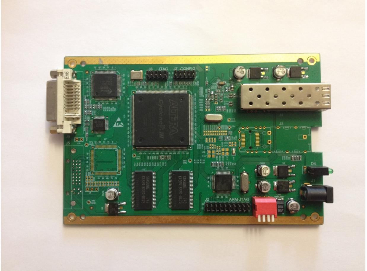
The Cyclone III board used on the receiver side.
