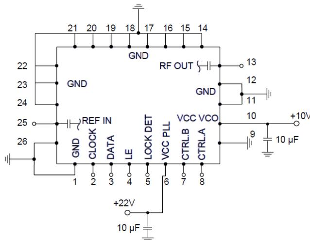
Figure 4.13.: The phase-locking loop circuit diagram.
