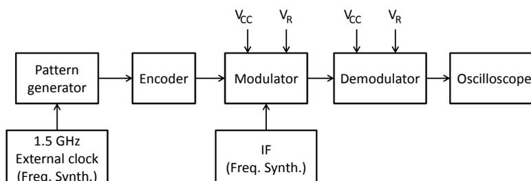
Figure 5.15.: Block diagram of baseband test setup.
