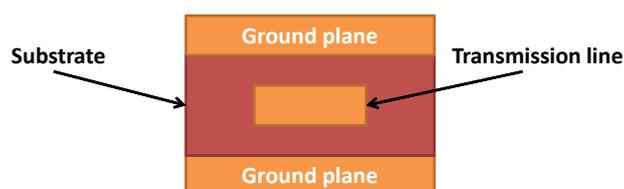
Figure 4.7.: Cross-section of a stripline.
