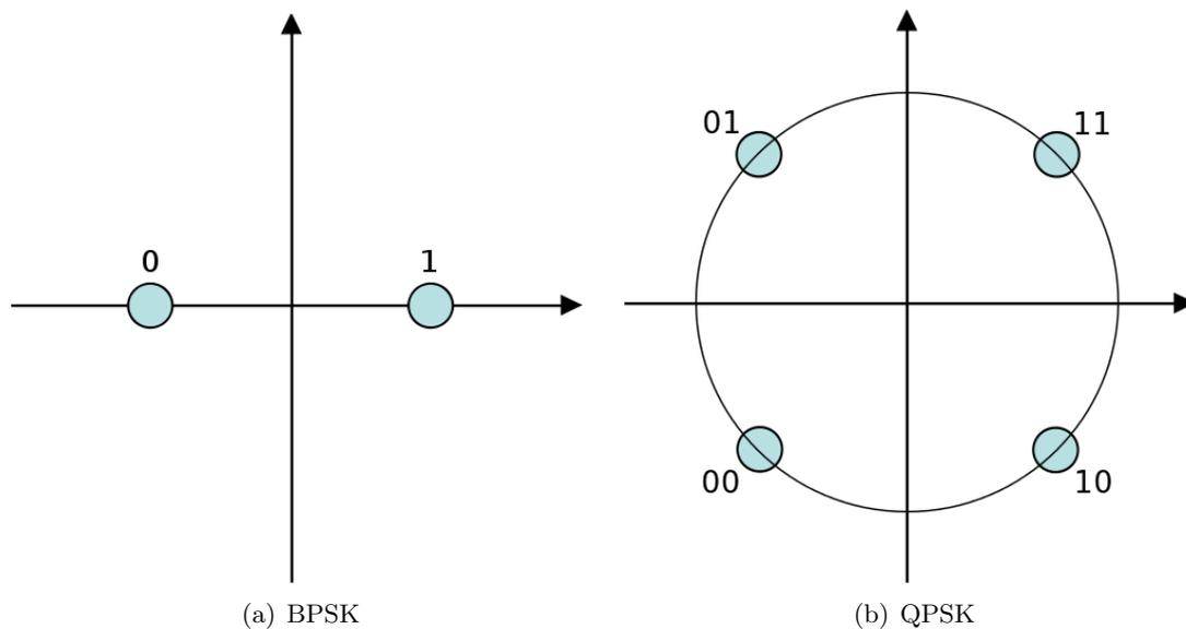
Figure 3.3.: Constellation diagram for BPSK and QPSK.
