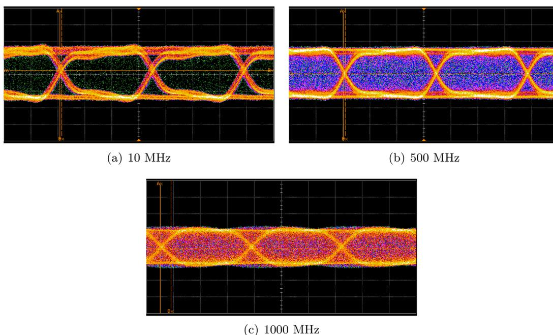
Figure 5.10.: Output from the baseband modulator for different intermediate frequencies.
