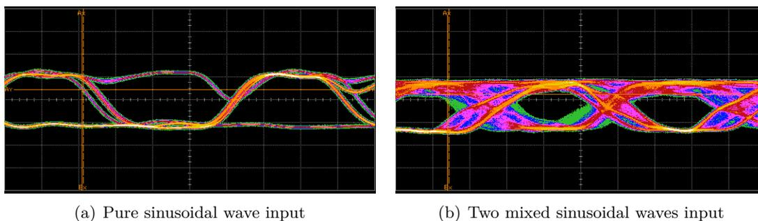
Figure 5.14.: Output from the demodulator for one and two sine waves.
