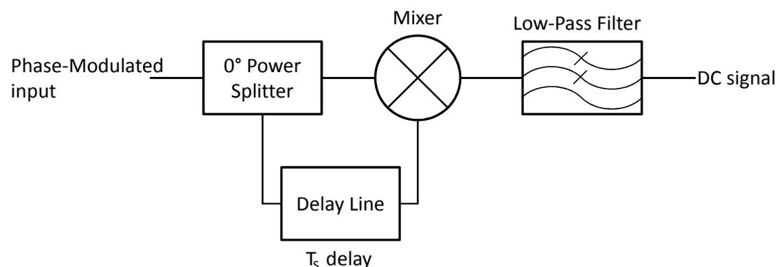
Figure 4.15.: A block diagram that shows the principle of the demodulator.
