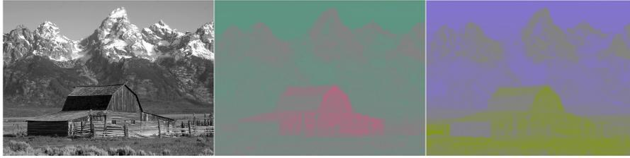
Figure 3.7.: An YCbCr-encoded image divided into luma, blue-difference and red-difference chroma components.
