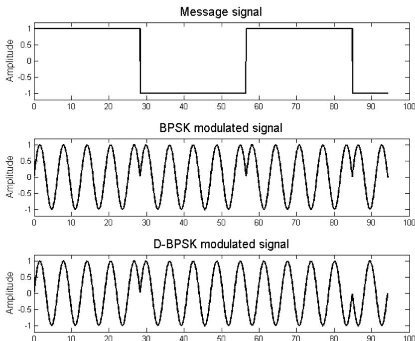
Figure 3.4.: The difference between BPSK and D-BPSK.
