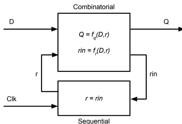
Figure 4.3.: Generic two-process circuit.
