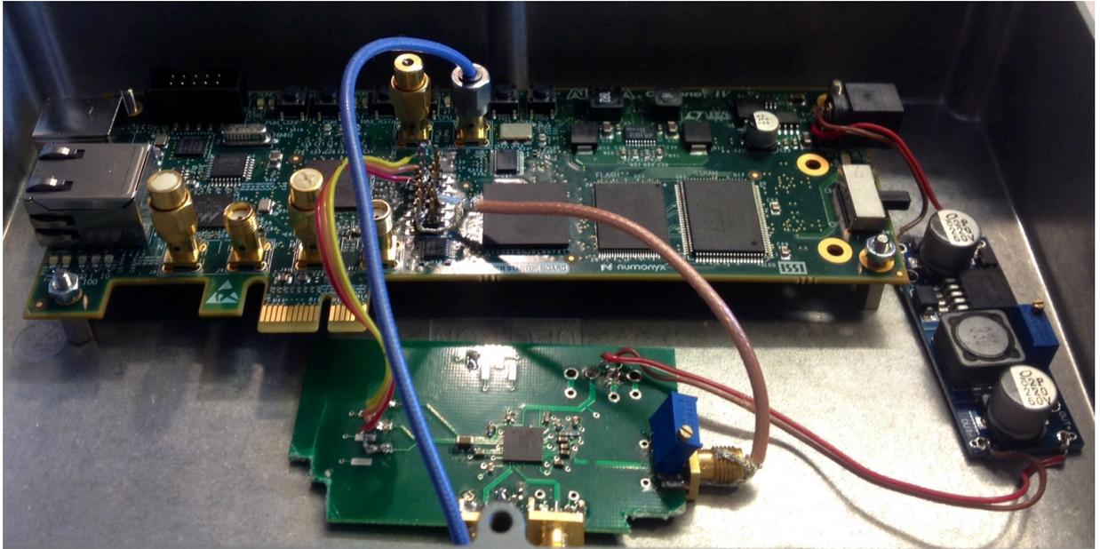
The Cyclone IV GX board with the clock conditioner and a power supply.
