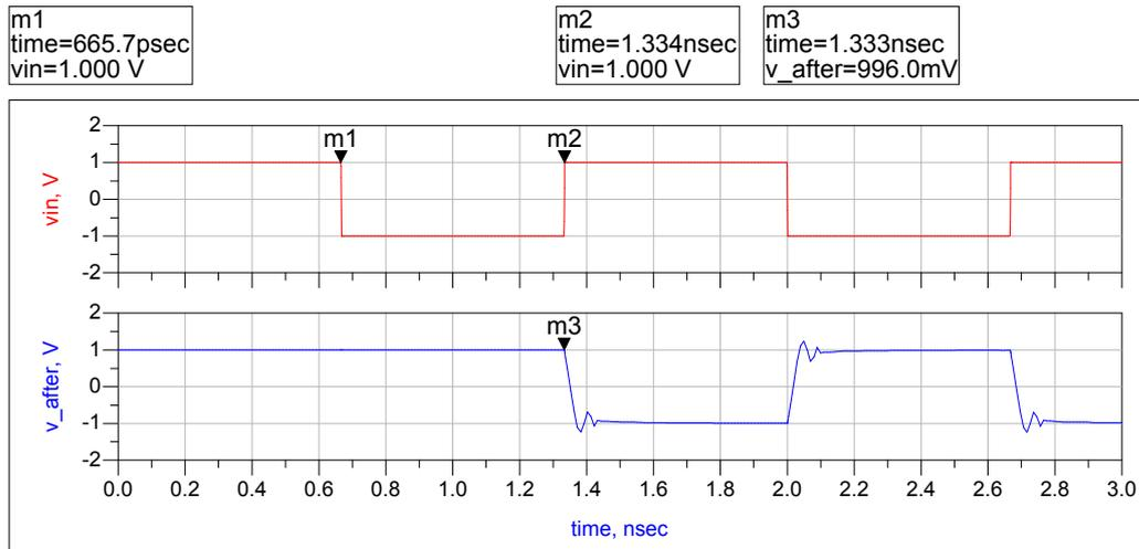
Figure 4.17.: The simulation results in ADS for the transient analysis.
