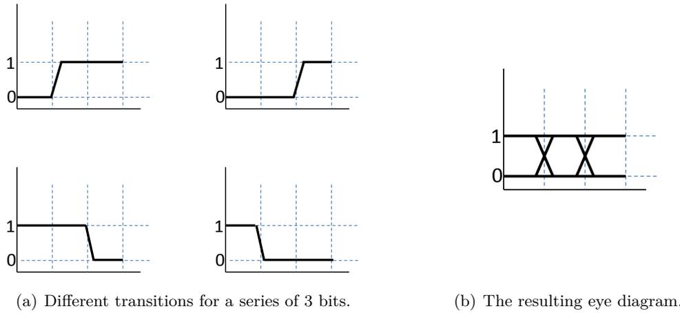
Figure 3.8.: The principle of an eye diagram.
