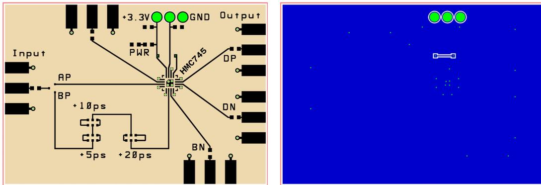
(a) The front of the first baseband demodulator. (b) The back of the first baseband demodulator.
