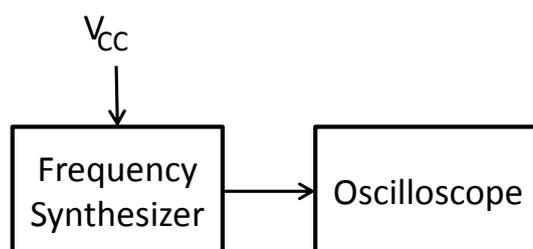
Figure 5.11.: Block diagram of frequency synthesizer test setup.
