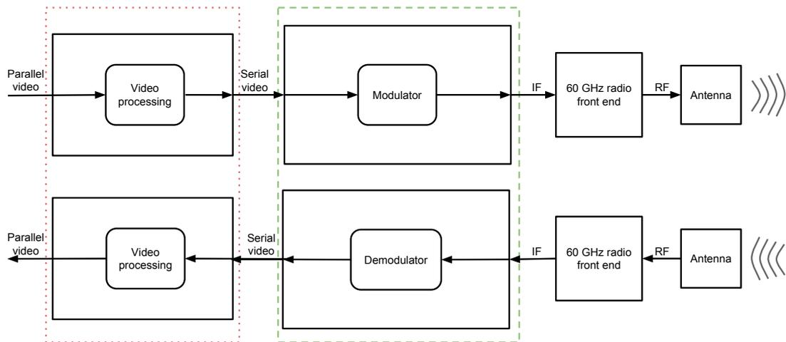
Figure 1.2.: An overview of the envisaged system. The red dotted box contains the video processing part and the green dashed box contains the radio baseband.
