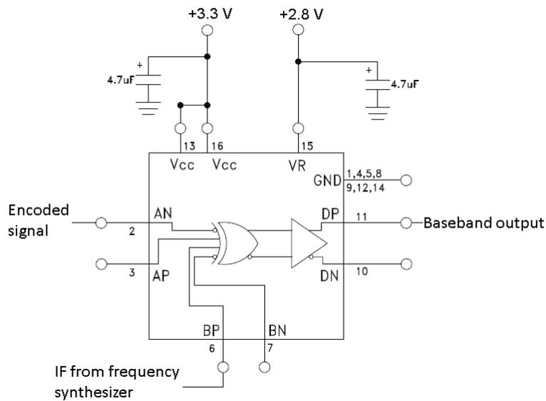
Figure 4.11.: Simplified circuit diagram of the baseband modulator.
