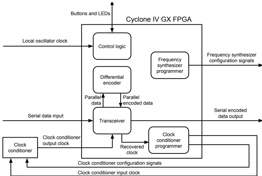
Figure 4.6.: A dataflow diagram of the most important signals of the FPGA design for the Cyclone IV FPGA together with the clock conditioner.
