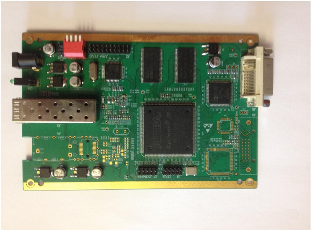
The Cyclone III board used on the transmitter side.
