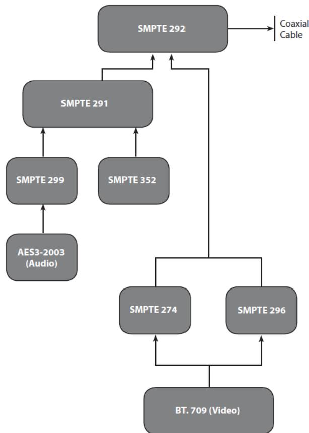
Figure 3.6.: A flow diagram describing the standards that are included in the SDI interface.
