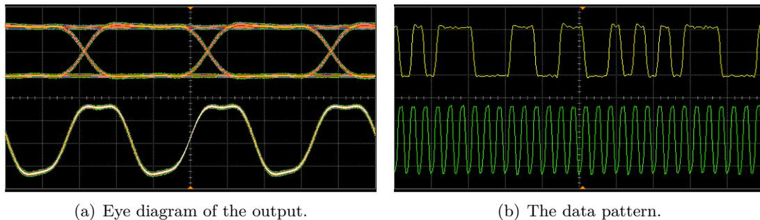
Figure 5.1.: Output from the pattern generator.
