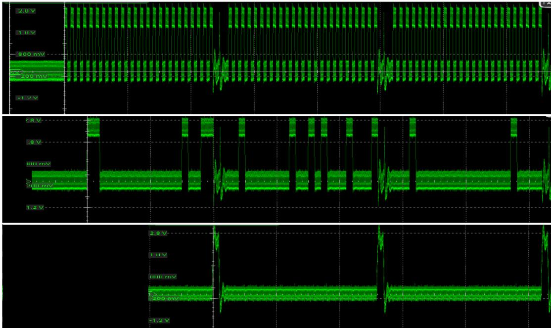
Figure 5.4.: Captures from the oscilloscope measurements of the frequency-synthesizer programmer output.
