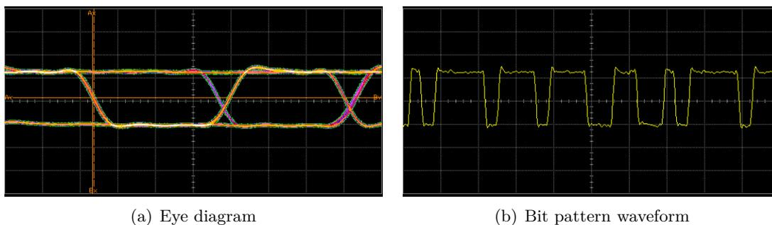
Figure 5.8.: The encoded data output from the transceiver.
