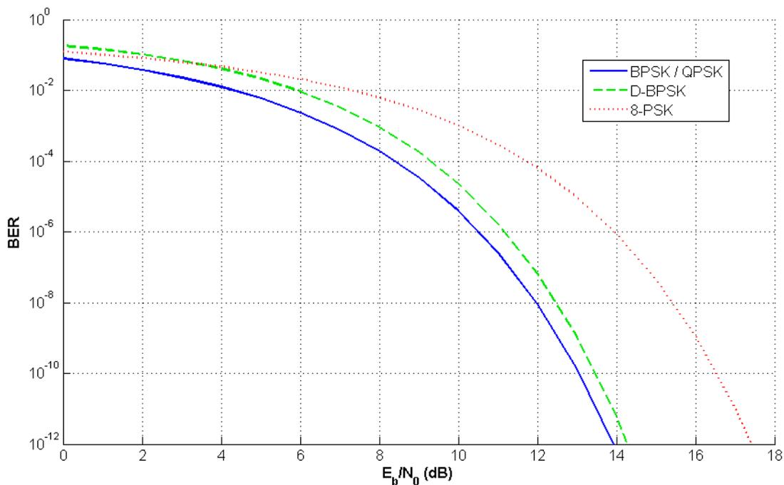
Figure 3.9.: BER vs  $E_b/N_0$  for different modulation schemes.
