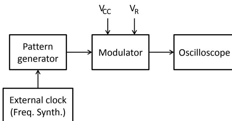
Figure 5.9.: Block diagram of modulator test setup.
