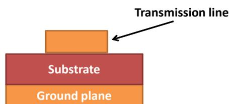
Figure 4.8.: Cross-section of a microstrip.
