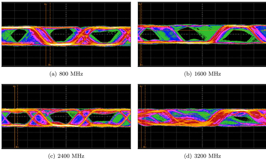
Figure 5.18.: Output from the baseband with terminated inputs and 3 dB attenuator for different intermediate frequencies.
