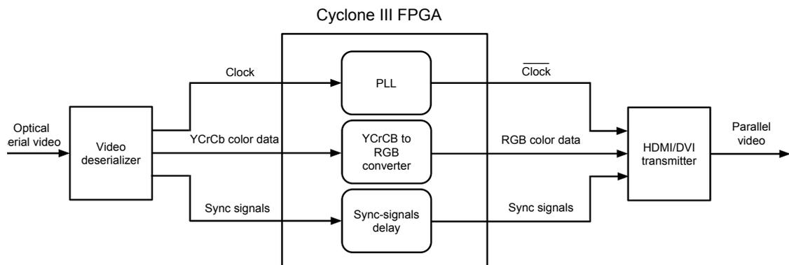
Figure 4.5.: Overview of the FPGA design for video processing on the receiver side.
