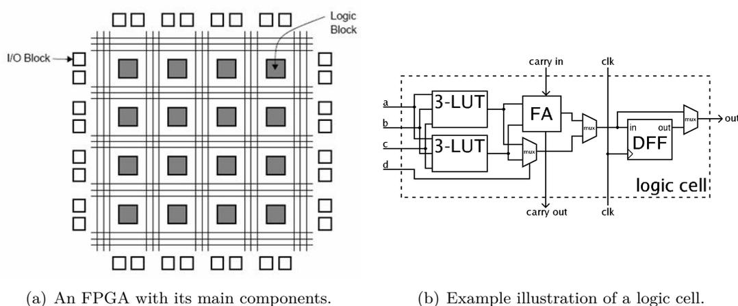
Figure 4.2.: Basic description of an FPGA and a logic cell.
