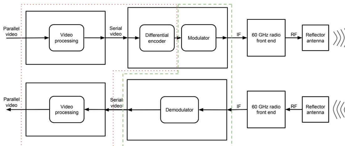
Figure 4.1.: Overview of the complete system. The red dotted box contains the digital parts and the green dashed box contains the analog parts.
