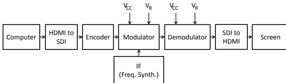
Figure 5.19.: Block diagram of video test setup.
