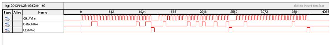
Figure 5.3.: Capture of the signals from the frequency-synthesizer programmer using Signaltap II.
