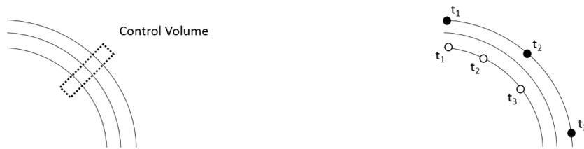
(a) Eulerian approach where the particles are monitored as they pass the control volume. (b) Lagrangian approach where every particle is continuously followed.  $t$  is time.
