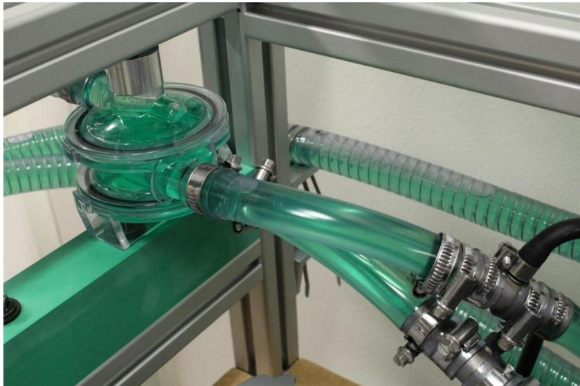
Figure 2: Separator mounted in test rig. In the lower right corner the connections for the pressure sensors are visible.
