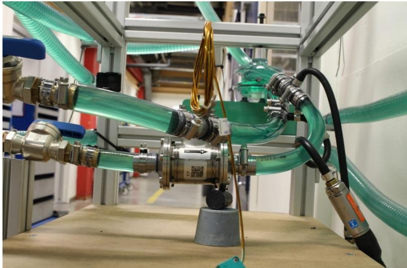
Figure 7: Hoses in the inner circuit leading up to the separator. Flow meter, temperature sensor and pressure sensors are connected to the circuit.
