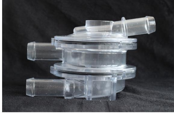
(b) Transparent separator model used in the experimental tests.
