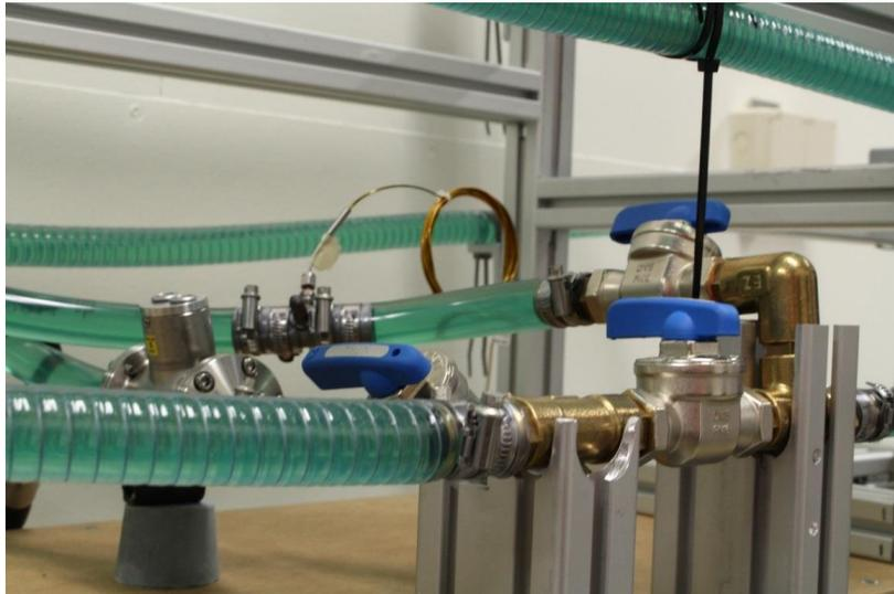
Figure 6: Valves to open and close the inner circuit.
