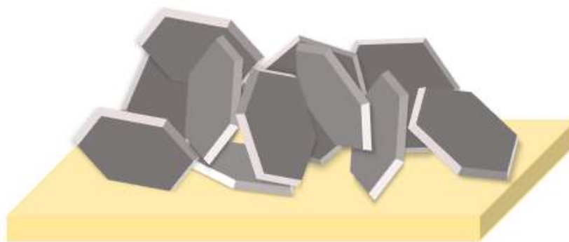
Figure 3.3: Typical deposition behavior of zinc onto an electrode surface.
