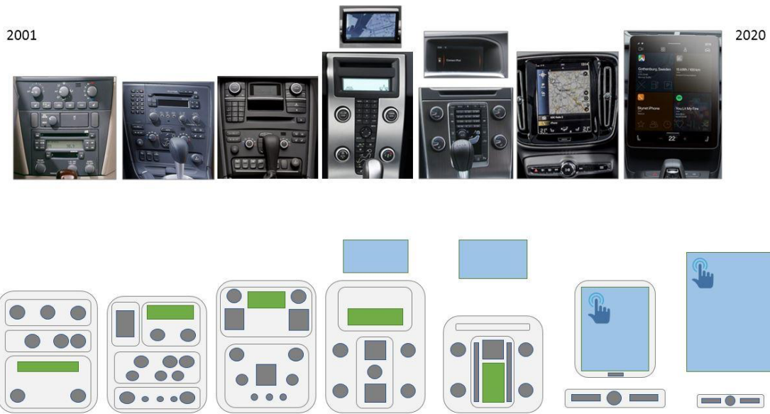
Figure 13. Transition of Volvo cars' IVI over twenty years (Image source from Volvo cars, graphical image by the author)
