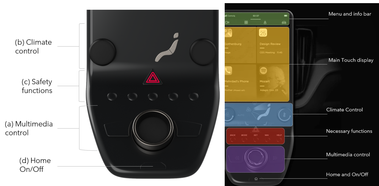
Figure 24. The commonly used functions as physical controls
