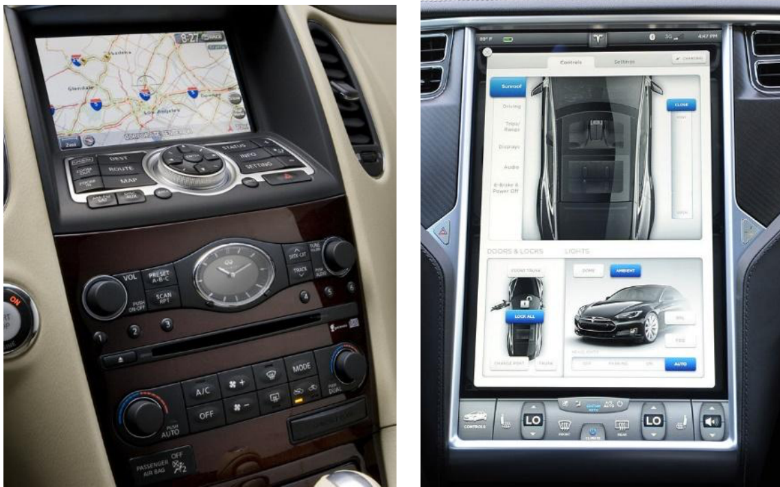
Figure 2. IVI with dedicated physical controls (Left- Infiniti), IVI with only one multifunctional touch display (Right-Tesla)
