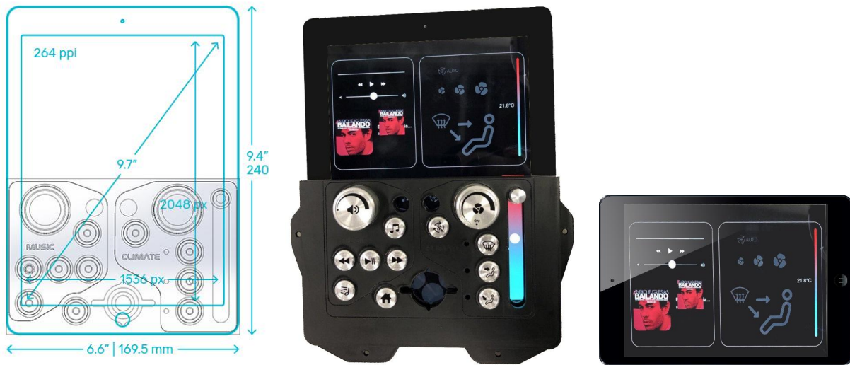
Custom made physical and digital HMI for user testing
