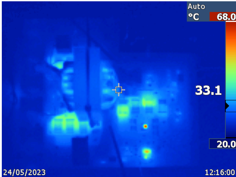
Figure 4.22: Temperature behavior of the converter with snubber at V_{in}=158 V, V_{out}=40 V and P=400 W
