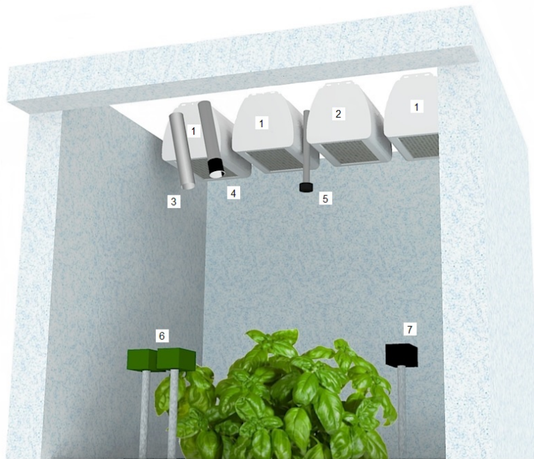
Figure 3.1: Front view of the experimental unit. 1) Background lamp. 2) Excitation lamp. 3) Fluorometer. 4) IR Radiometer. 5) Maya2000 Pro. 6) JUNIOR-PAM. 7) JAZ.
