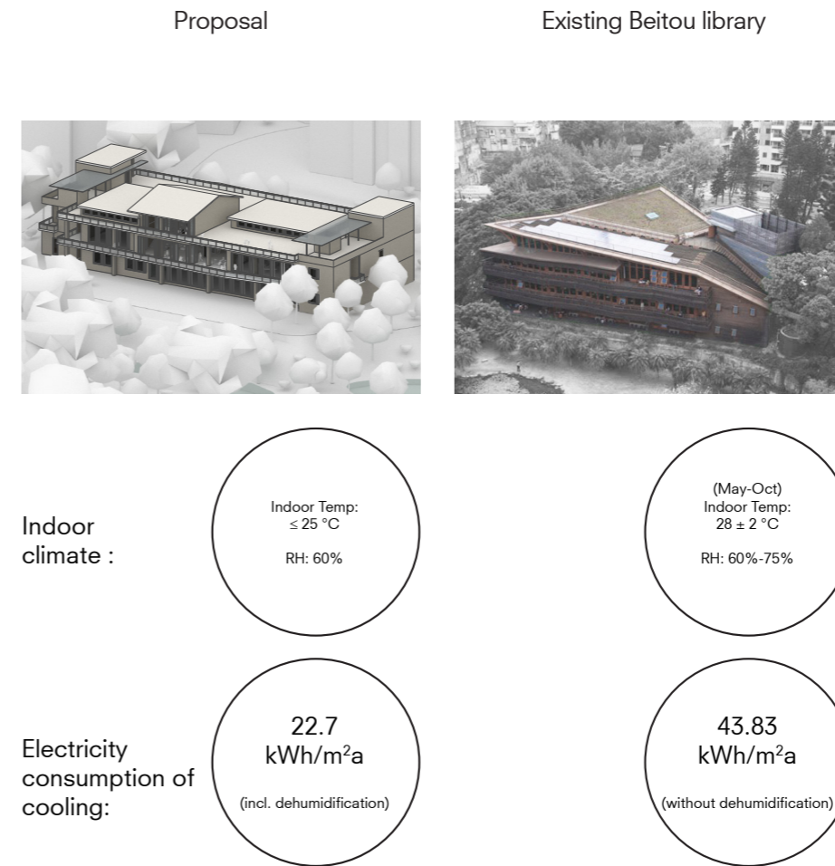
Fig. 65 Energy performance of Cooling and dehumidification
