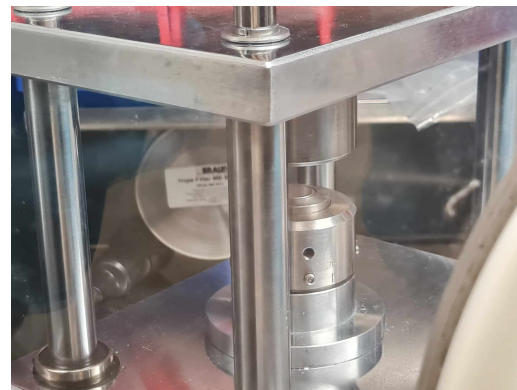
Figure 3.6: The figure shows how a manual hydraulic press was used to enclose the active material and separator within the battery enclosure. The press was also placed within the argon filled glove box.
