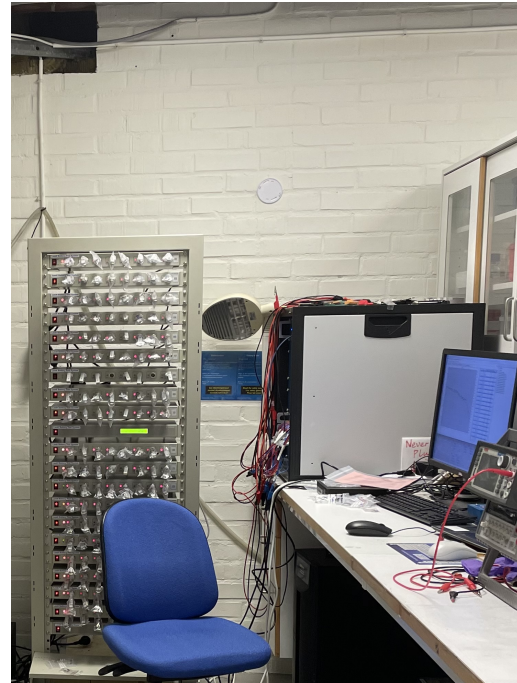
Figure 3.8: Landt battery testing machine
