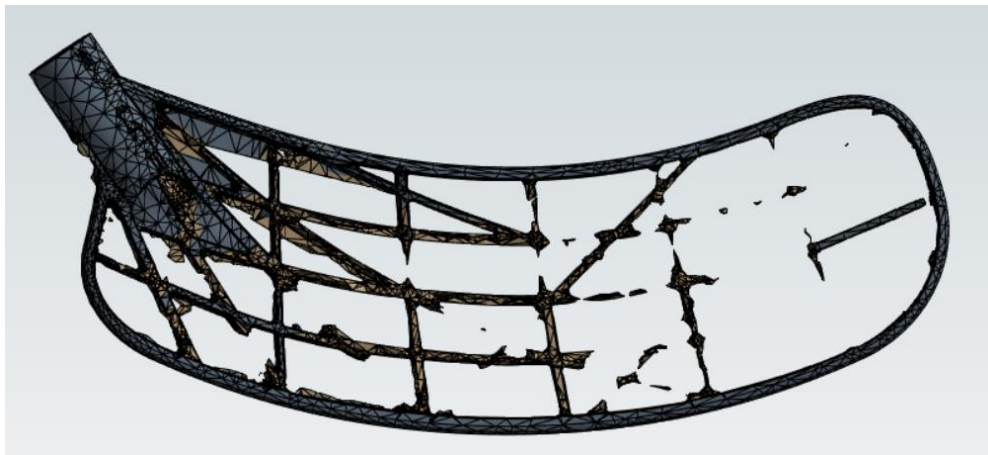
Figur. 12- Topology optimizing Evolite
