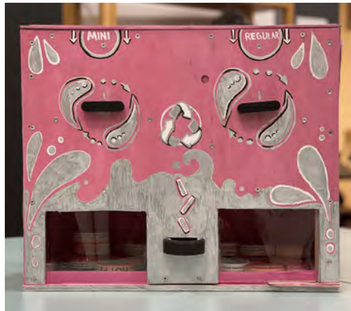
Figure 5.7: Gacha Machine prototype ready for alpha testing. Image taken by the authors.
