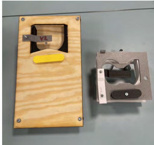
Figure 5.5: Version 1 (right) and Version 2 (left) of turning mechanism for Gacha Machine prototype. Image taken by the authors.
