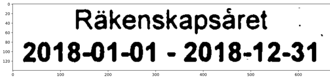
(b) Reference text after being passed through an opening filter with kernel size s = 3 , and then a median filter with kernel size s = 5 . Almost all noise has been removed, but the corners are not as sharp as before.
