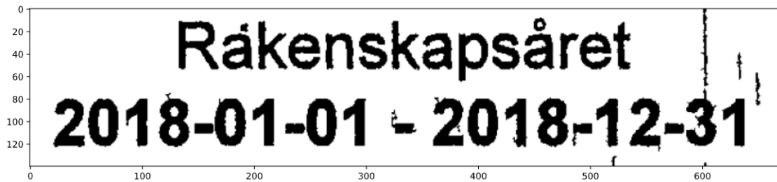
(c) Reference text after being passed through an RCC filter with cutoff size = 40 . Most of the noise is removed, but a few streaks remain. The filter also removes one dot above the \ddot{a} and leaves some characters, especially numbers, with rough edges.
