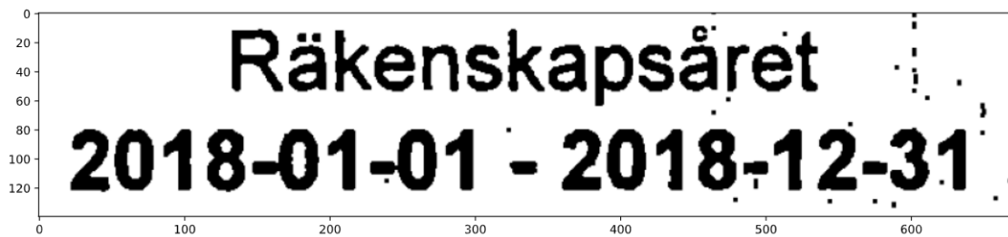
(c) Reference text after being passed through a median filter with kernel size s = 3 , and then an opening filter with kernel size s = 3 . Some noise remains in the image.
