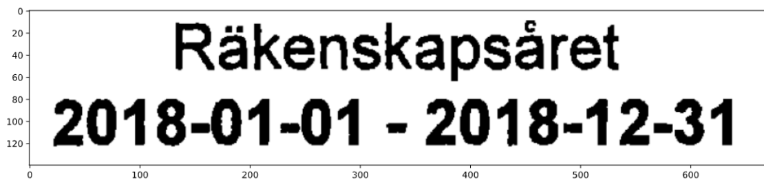
(d) Reference text after being passed through an opening filter with kernel size s = 3 , and then a RCC filter with cutoff size = 25 . No noise remains in the image, and the text is not noticeably distorted.
