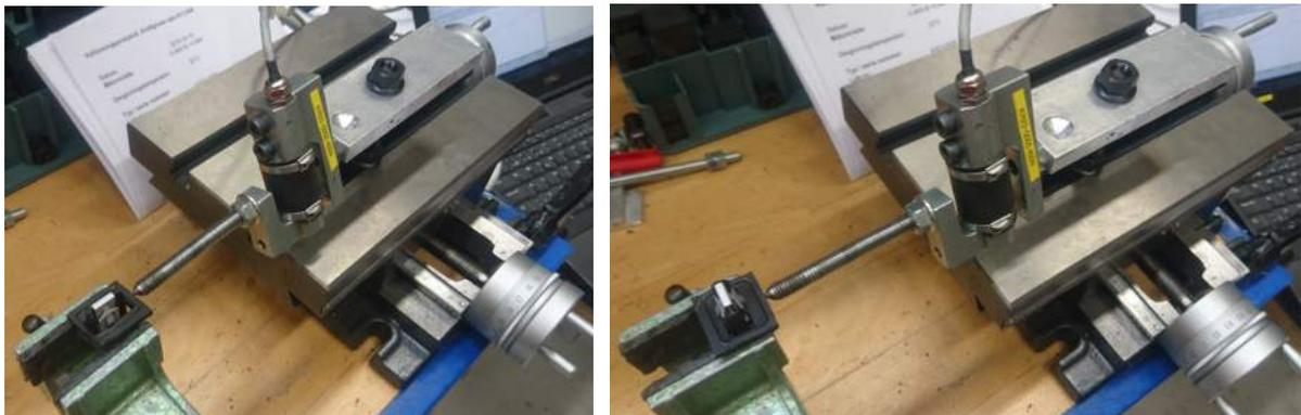
(a) *The test configuration for friction test.* (b) *The test configuration for measurement of stiffness in y-direction.*
