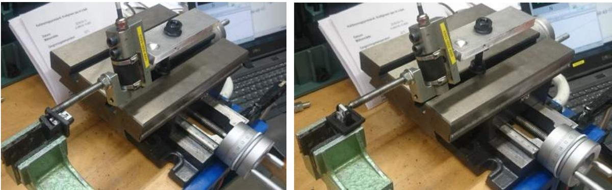
(a) The test configuration for measuring the rotational stiffness around the y-axis. (b) The test configuration for measuring the rotational stiffness around the z-axis.
