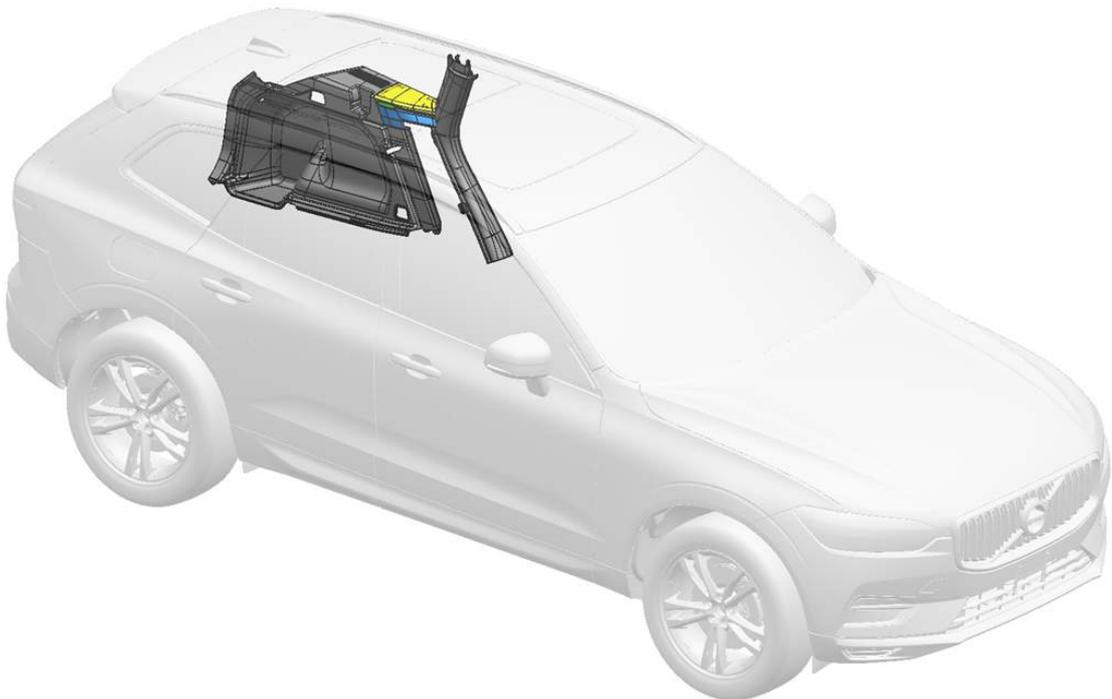
Figure 1.1: *Example of parts connected with the studied clip.*
