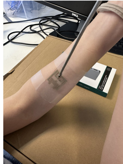
(b) Use SMA to test the stencil printing antenna
