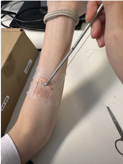
(a) Use SMA to test the copper tape antenna
