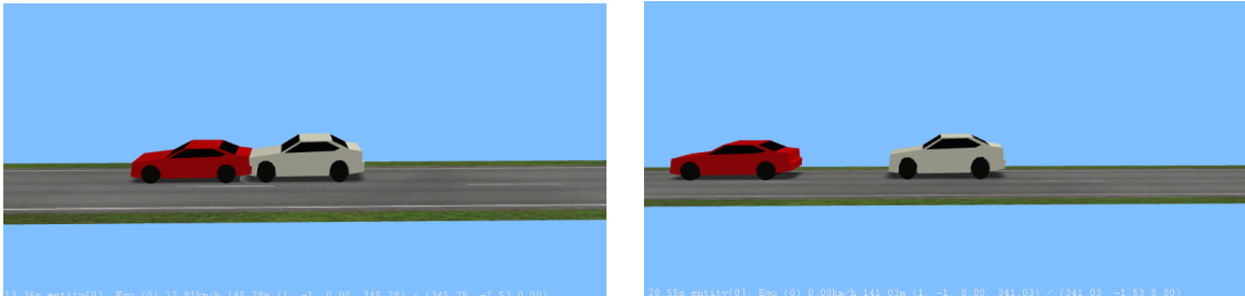
(a) Simulation of AEB activation at TTC = 0.96 s for a deceleration level of -9.27 m/s 2 .
