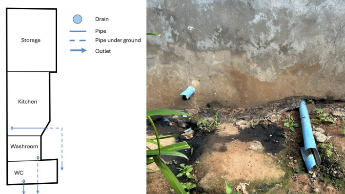
Figure 5.6: Left: Plan view of utility building with water pipes and outlets. Right: outlets outside the utility building from washroom (right pipe) and bathroom (left pipe)
