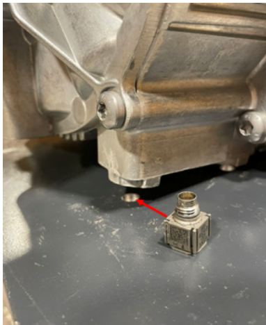
Figure 2.16: Measurement of interface locations is limited due to the accessibility of transducers.
