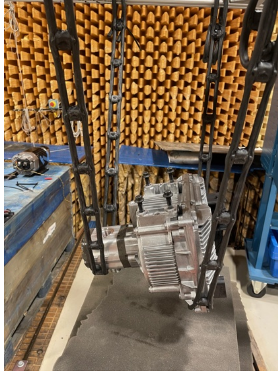
Figure 3.4: EHPS suspended via bungee in Free-free condition
