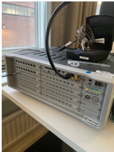
Figure 3.3: Siemens SCADAS frontend
