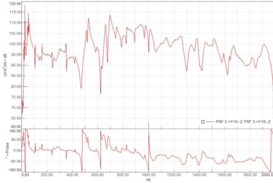
Figure 2.3: Frequency response functions have a magnitude and phase component
