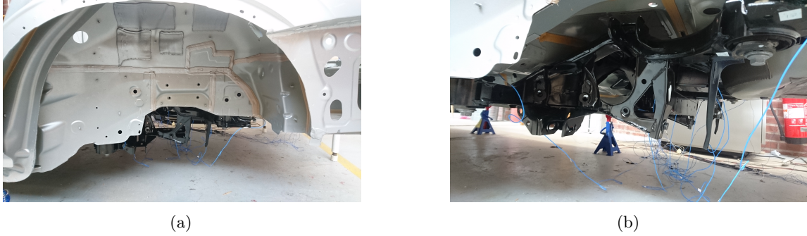
Figure 3.8: The assembled rear subframe on the BIW. (a) Attached rear subframe on the BIW from the side. (b) attached rear subframe on the BIW from below. Some of the triaxial sensors as well as one of the four M14x110 bolts including the washer is shown in (b).
