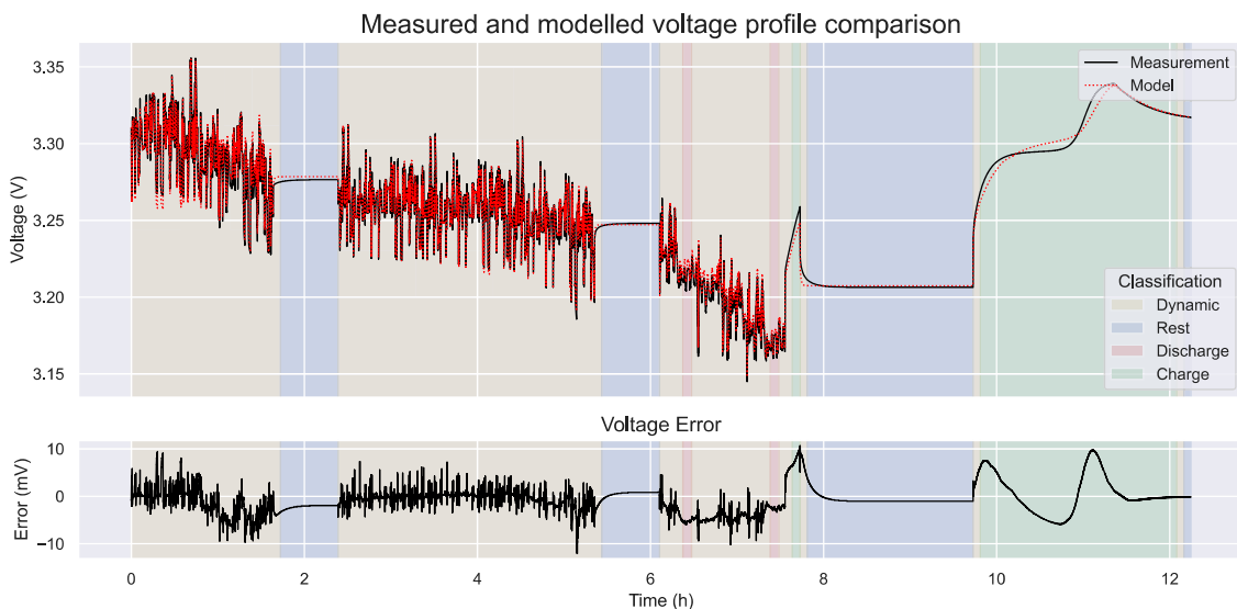
Figure 4.1: Voltage profile from PyBaMM (measurement) and as generated by the ECM, with corresponding errors. This voltage profile is generated by the ECM based on the current state–space formulation.
