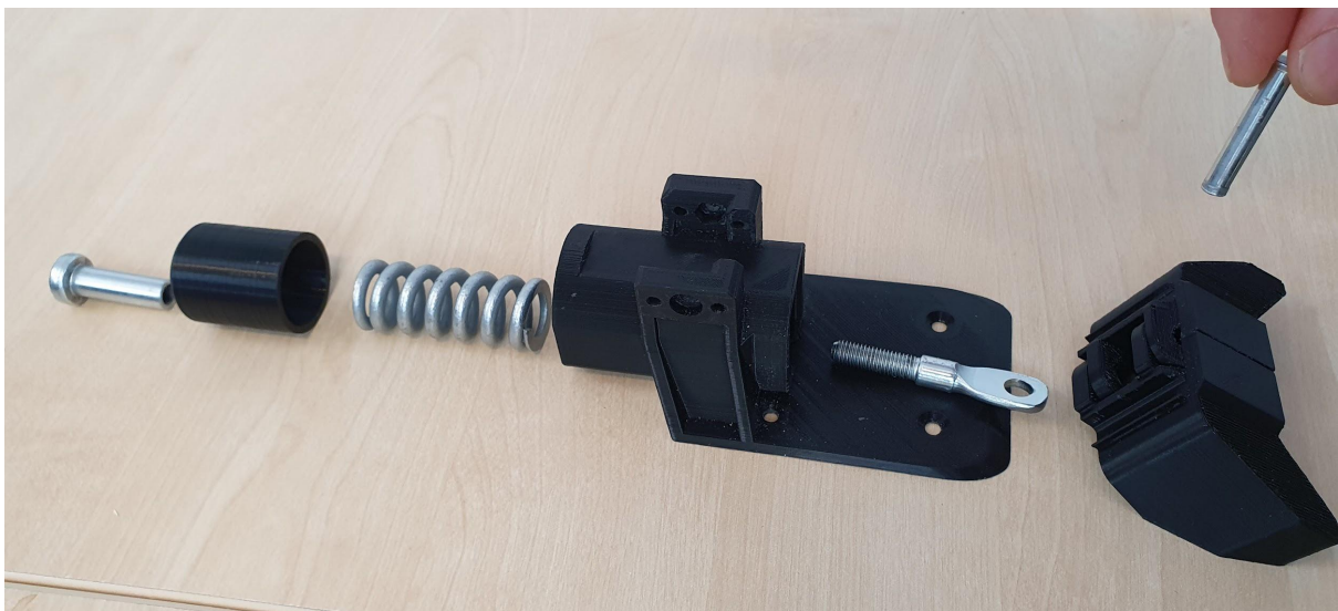
Figure 5.24 Exploded view of the alpine assembly. (Authors' image, 2022)
