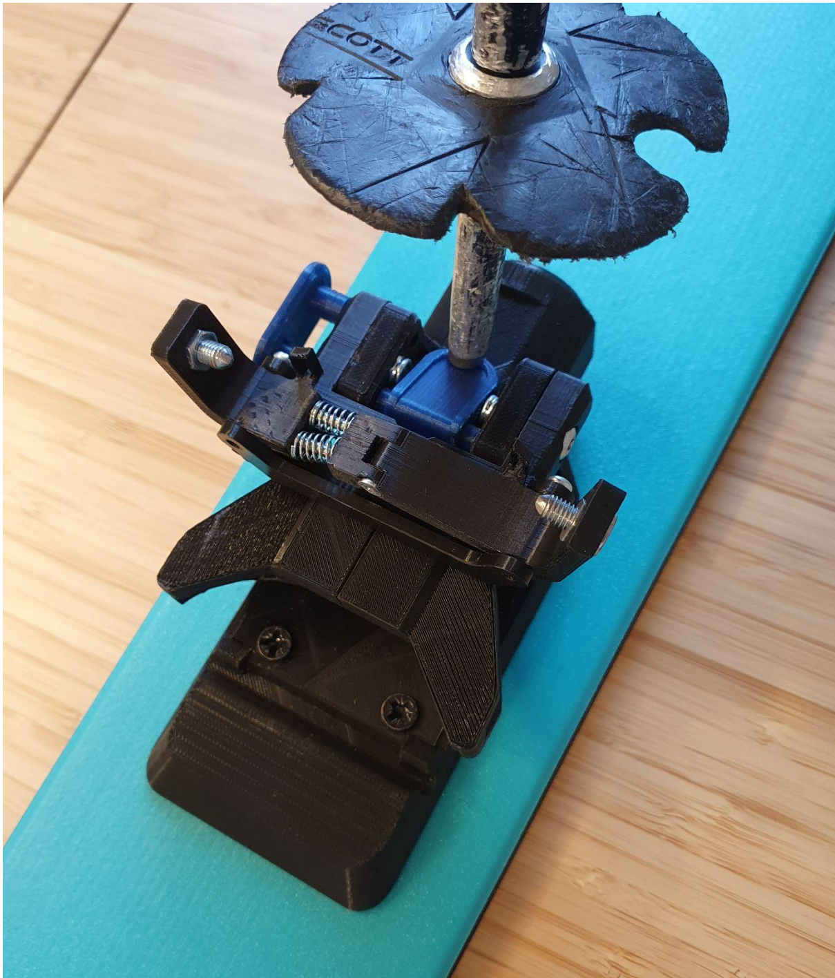
Figure 5.21 Centered lever with a fixed position. A lever that was not attached to the jaws could provide leverage beyond the rotation point used for rotating the whole tech toe. (Authors' image, 2022)
