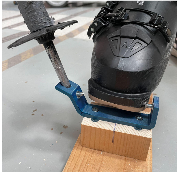
Figure 5.14 U-bracket . Testing of a flexible bracket prototype. (Authors' image, 2022)
