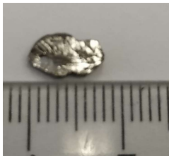
Figure 12: Crystal piece of Mn_3Sn after being broken with a hammer to the left. Crystal after being polished and with attached Hall contacts with platinum wires on the right.
