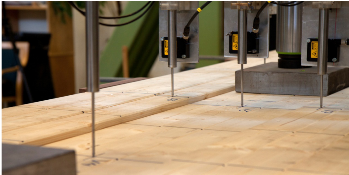
Figure 6.4 Close-up of sensors and load plate on one of the narrow SLT deck specimens, clearly displaying interlaminar slip in laboratory tests by Ekholm (2012).
