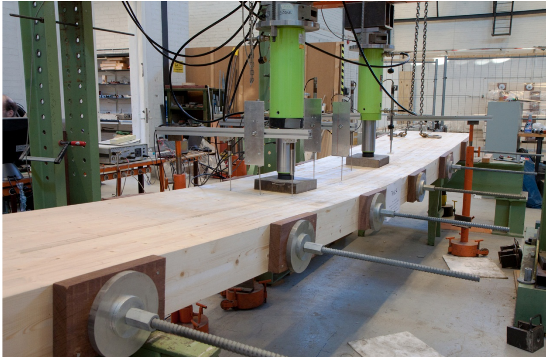
Figure 5.1 Setup of experimental testing of a narrow SLT deck at Chalmers, Ekholm (2012).
