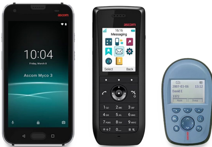
Figure 2.1: An Ascom smartphone, DECT phone and pager. Mobilenheter för vården [Image], by Ascom (n.d.-g) 1 .
