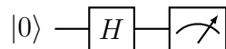
Figure 2.1: A simple, single-qubit quantum circuit that places a qubit into a superposition using a Hadamard gate, and then measures its state. The measured state has equal probability of being 0 and 1.
