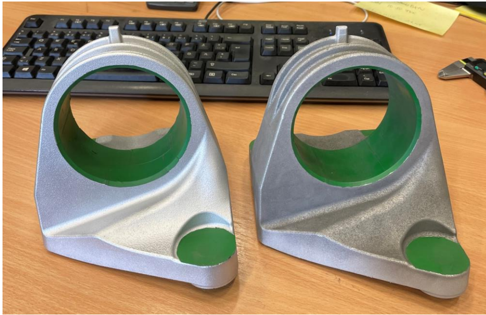
Figure 2.19: Powertrain suspension bracket after (left) and before (right) surface treatment with glass blasting.
