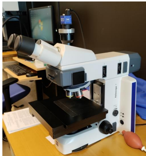
Figure 2.9: Zeiss Axioscope 7 used for imaging the microstructure and porosity.
