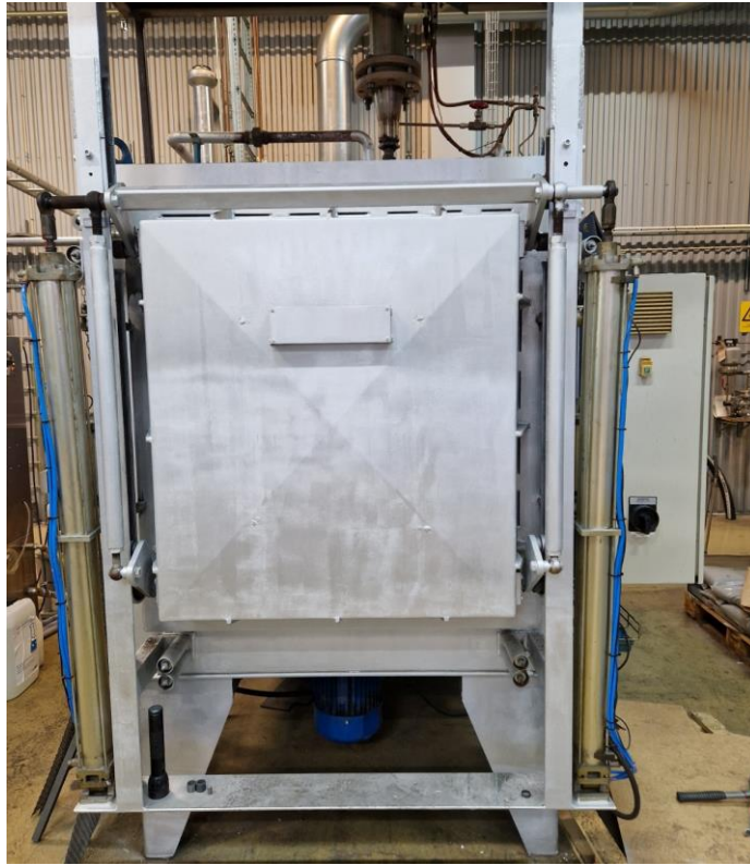
Figure 2.13: Nitriding furnace at Hårdservice used for heat treatment of the build plate.
