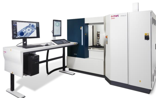
Figure 2.12: Comet Yxlon FF35 CT scanner (From [13]).
