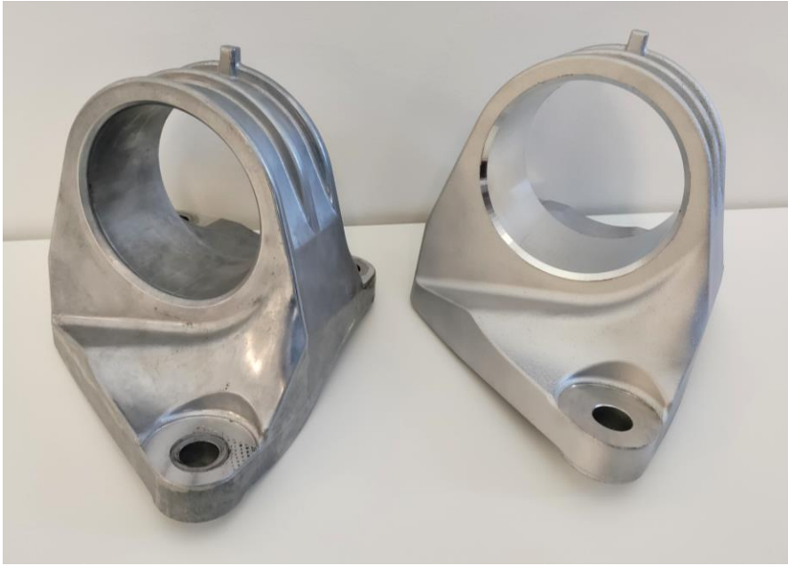
Figure 2.21: Production HPDC bracket (left) and post-processed 3D printed bracket (right).
