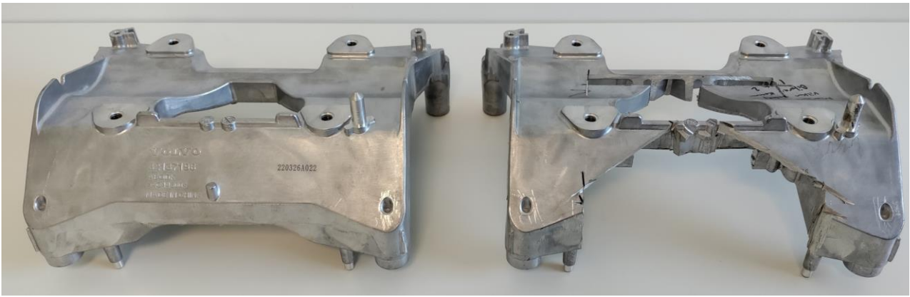
Figure 2.4: HPDC part used for tensile samples. Original part on left, part with samples cut out on right.
