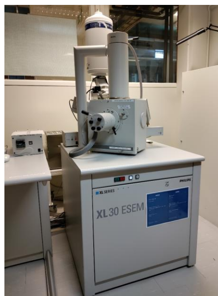
Figure 2.10: Philips XL30 ESEM Used for imaging the microstructure.
