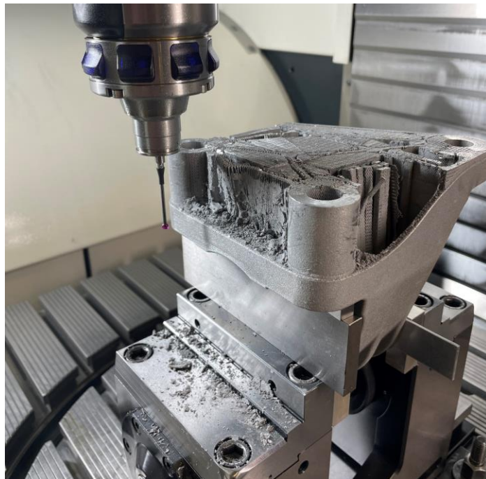
Figure 2.18: Powertrain suspension bracket mounted upside down for support removal.
