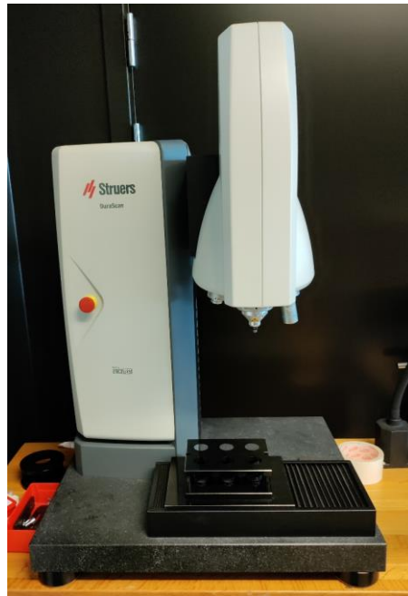
Figure 2.6: Struers DuraScan microhardness tester used to measure hardness.
