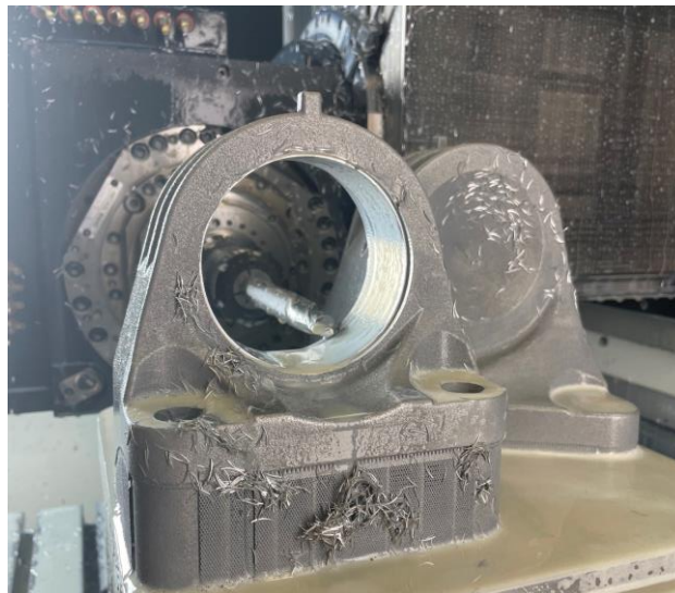
Figure 2.16: Central hole of powertrain suspension bracket being milled out.
