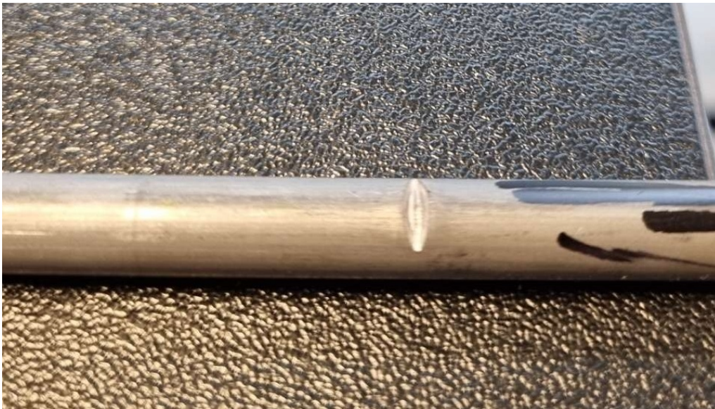
Figure 3.1: Photograph of notched sample.
