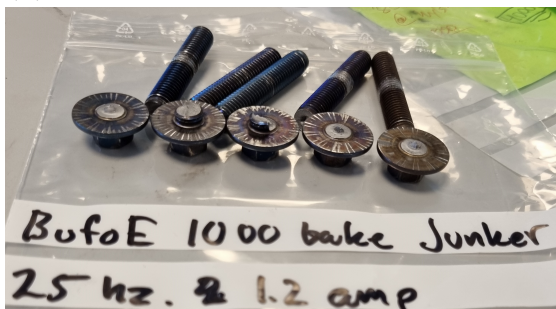
(c) Bake hardened BUFOe 1000 fractures.
