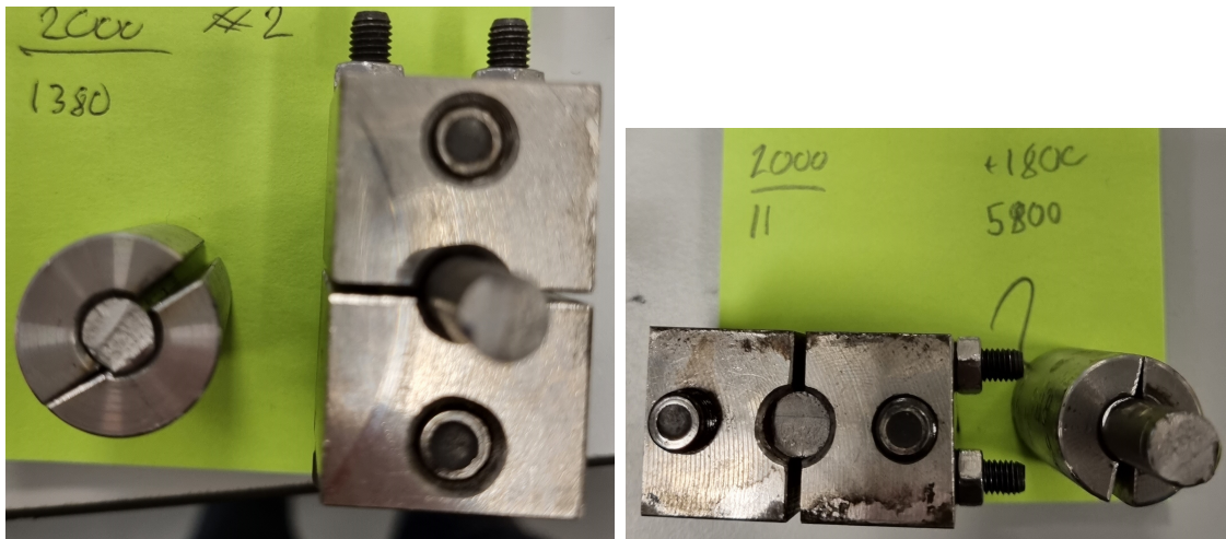
(a) Fracture at bisected cylinder grip. (b) Fracture at rear grip.
