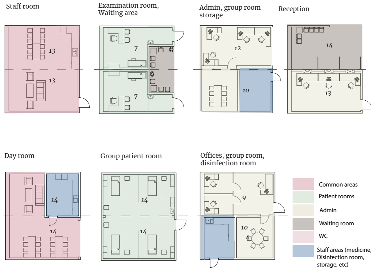
Diagram. Different ways of combining modules of kind B or C
